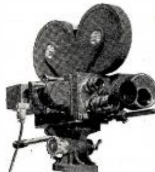
**THE MAURER 16MM.**, designed specifically for professional use, equipped with precision high-power focusing and view-finder. Standard equipment includes: 235° dissolving shutter, automatic fade control, view finder, sunshade and filter holder, one 400-foot gear-driven film magazine, a 60-cycle 115-volt synchronous motor, one 8-frame handcrank, power cable and a lightweight carrying case.
