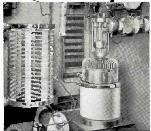
Federal's F-892-R installed in Power Amplifier
