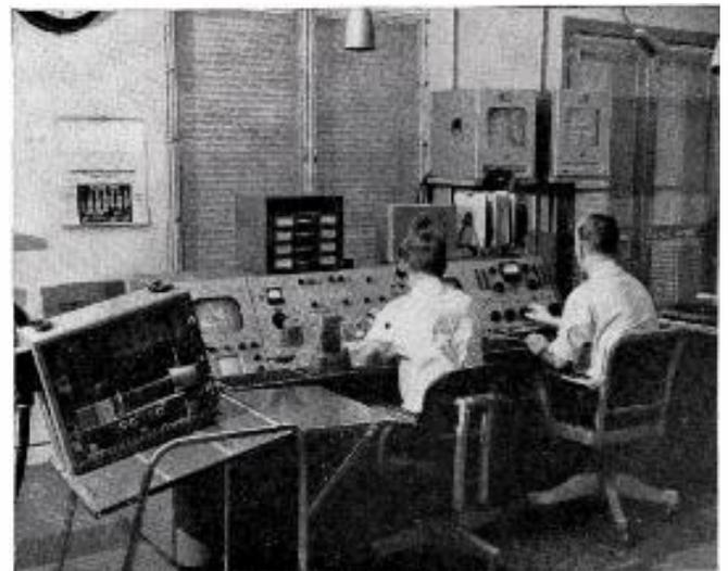
Two engineers control WNAO's entire program schedule, film, studio and network—with Federal Transm Control Console and Poly-Efex Scanner providing complete transmitter supervisory control and audio/video switch. Scanner includes 2 slide sources, four-channel video switch and "special effects" section.
