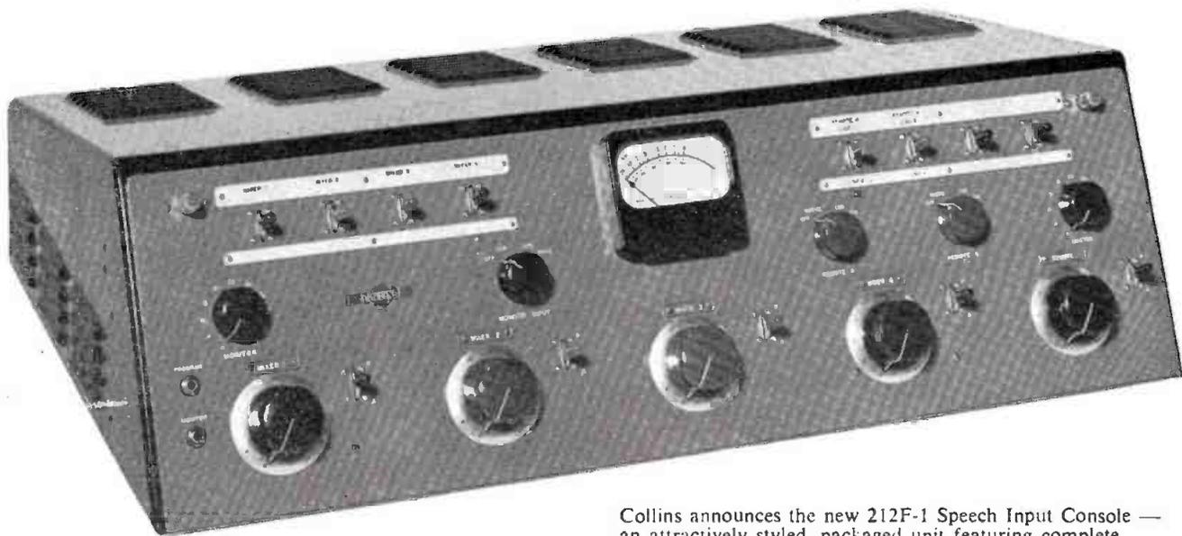
Collins announces the new 212F-1 Speech Input Console — an attractively styled, packaged unit featuring complete flexibility. It provides complete control over simultaneous broadcasting and auditioning from any combination of three out of eight possible inputs. The addition of two pre-amplifiers provides for mixing five of twelve possible inputs. The 212F-1 also provides for monitoring of program, audition, or remote lines, and control of speakers and warning lights.
