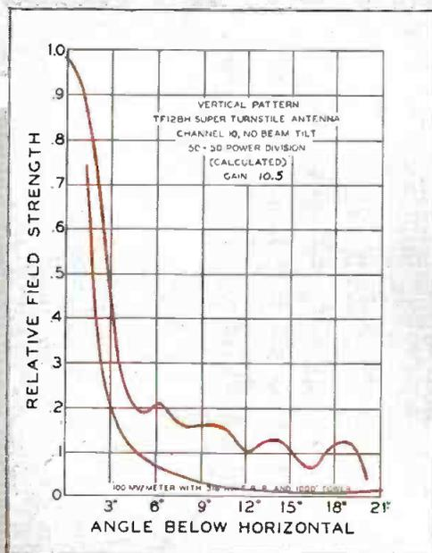
Vertical Field Pattern of new RCA TF-128H 50-kw antenna. Note complete absence of vertical nulls. Operated in conjunction with an RCA 50-kw TT-50AH transmitter, this antenna will "saturate" your service area with strong signals.
