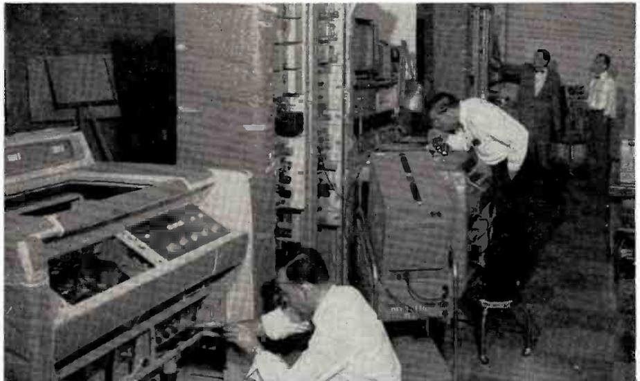
FINISHING touches are put on the first videotape recording-playback machines to come off the Ampex Corp. assembly line in Redwood City, Calif., fulfilling a production schedule announced seven months ago. KING-TV Seattle and KGW-TV Portland, Ore., got two of the
