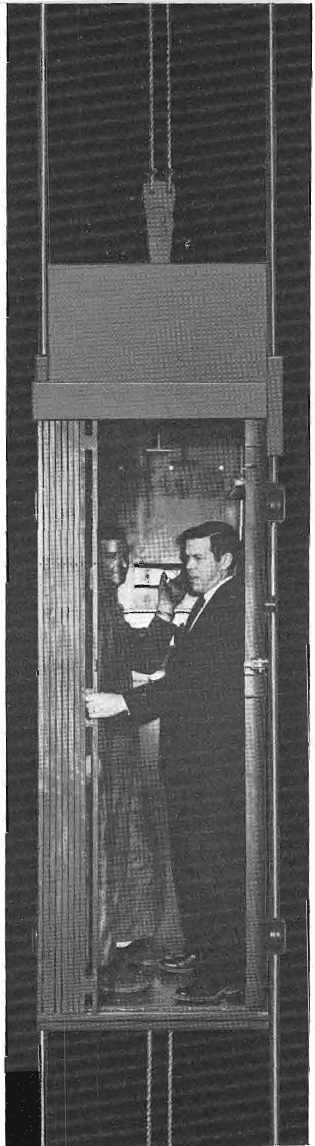
(right) Rated for a load of 750 pounds, will comfortably accommodate two people. Car stops automatically if door is opened, will not start until it is closed. Supported by a double set of cables, either one of which will hold the car and its full load.
