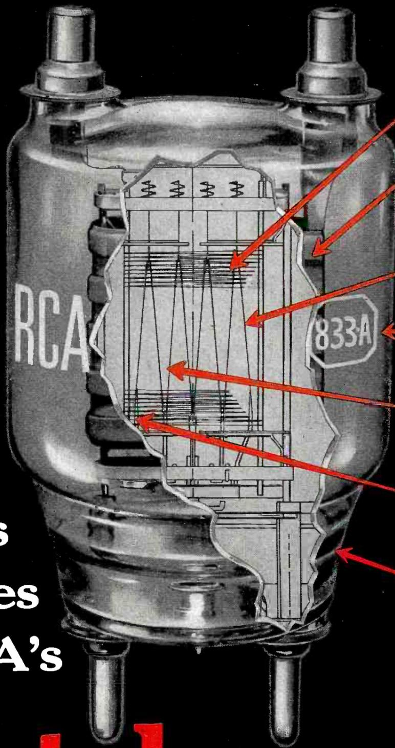
**GRID**... Zirconium-sprayed to minimize grid emission.
