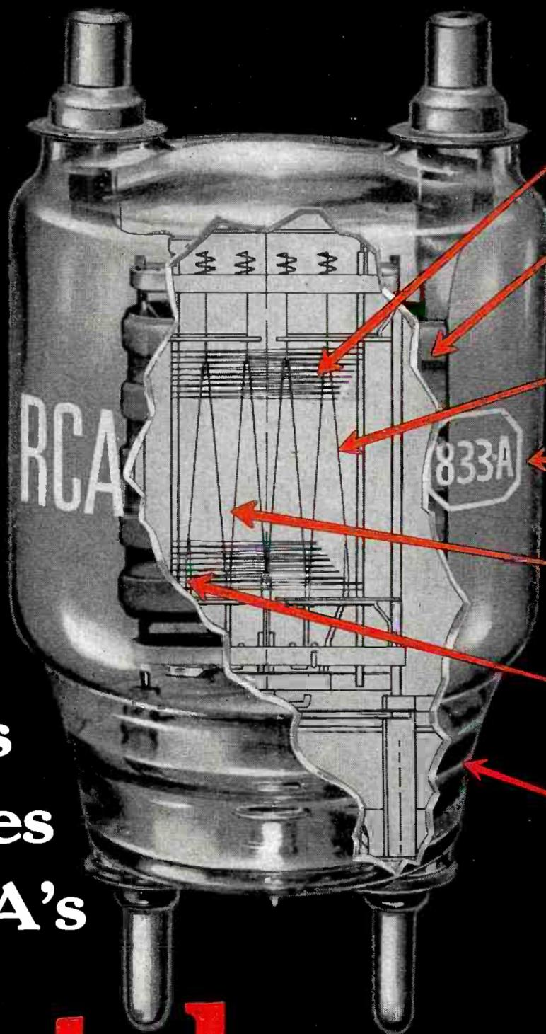
**GRID**... Zirconium-sprayed to minimize grid emission.
