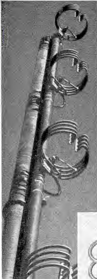
Above. Four sections of a BFA FM Antenna pole-mounted and interconnected by 3\frac{1}{4} " coaxial transmission line.
