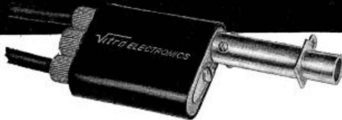
This self-normalling jack is for use in applications where a "normal-through" condition is known to be of a semi-permanent nature. It accepts a Nems-Clarke 966-A or 967 series patch cord plug for sampling or temporary re-routing. So used, the rear jack connection is automatically terminated to 70 or 50 ohm impedance. Removal of
