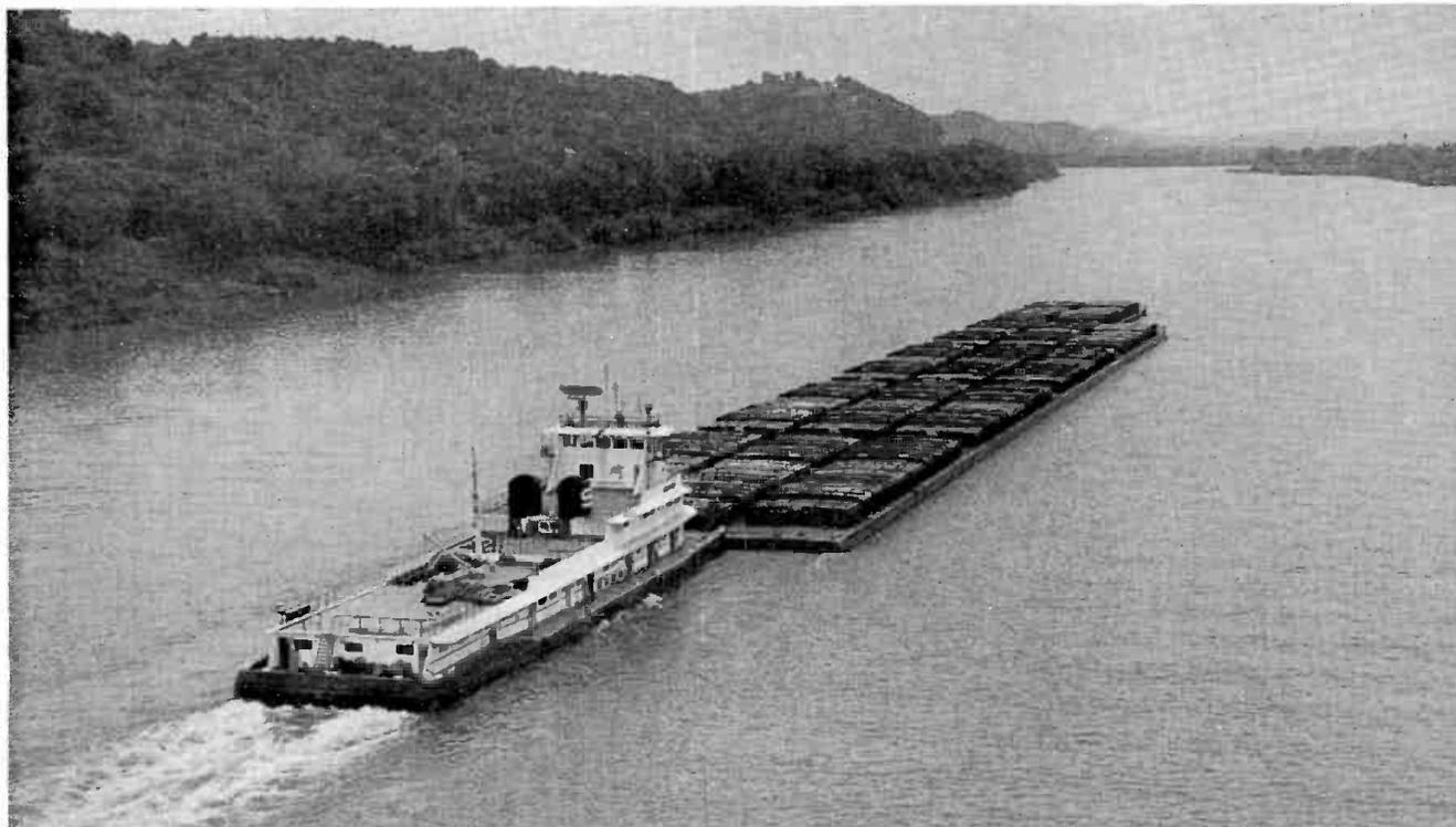
Fourteen 195 x 35 foot barges carry 21,000 tons of alumina up the Ohio to the Olin Mathieson Chemical Corp. plant
