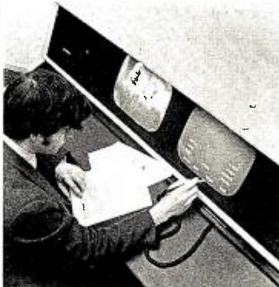
As explained by CMX Systems the editing and assembly processes permit either video tape or film to be edited electronically "with equal ease and a higher level of artistic flexibility than any previous editing system." The CMX 600, an instant image-access system, automatically assembles broadcast-ready tapes to take maximum advantage of economies inherent with "high picture quality two-inch tape."
