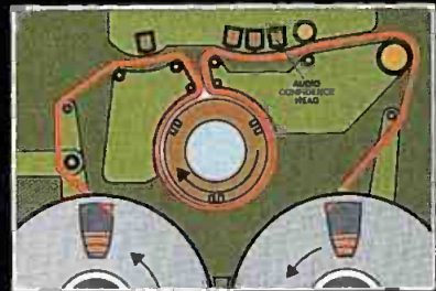
• Full audio and video confidence • "PRO" tape path reduces dropouts
