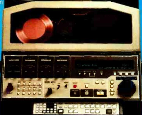
fast/slow motion range that provides real-time reverse and field/frame still motion. Plus programmable time compression up to 20%, with 0.1% accuracy.
