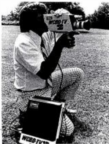
Beyond film. Quarter-inch videotape is the only mode for WCBD-TV Charleston, S.C., whose 22-lb. Akai minicam has completely replaced film.
