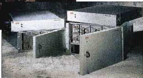
Perpetual transformation will continue to characterize the television plant beyond the "digital era." Racks of VTRs like these D-2 machines will ultimately yield to "digital video servers." The BTS Media Pool (r) provides time-scalable (10 minutes to hundreds of hours) video recording using RAID technology. In time, these systems will be low-cost enough to replace VTRs in most playback and distribution applications.
