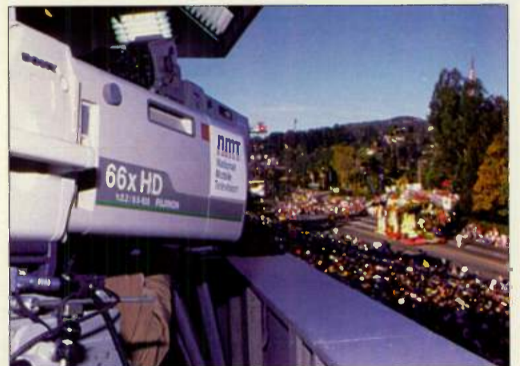
KTLA used a Sony HDC-700 camera with a 66X Fujinon lens.
