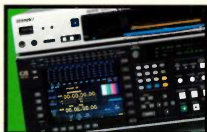
Sony's new HDCAM-SR VTR can record up to 600 Mb/s, with 450 Mb/s dedicated to video.
