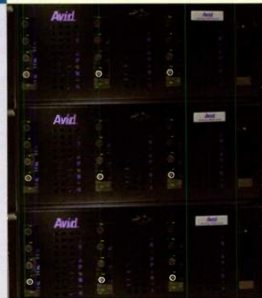
Avid's MEDIAArray ZX provides close to 3 TB of storage and has software that identifies problems in the storage subsystem.
