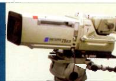
Sony's HDC-910 camera has an HAD image sensor that gives it low-light sensitivity.
