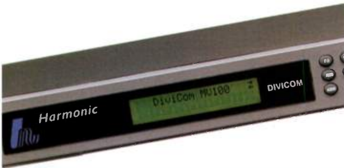
Harmonic's next-generation encoders are helping operators offer more VOD streams per QAM by achieving the same picture quality at a lower data rate. Movies today are generally encoded at 3.75 Mb/s, allowing for 10 VOD streams on a 256-QAM cable channel, but Harmonic says that data rates can be driven much lower, even for sports programming.
