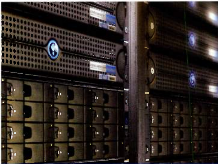
Network-based DVR systems that rely on headend video servers, such as this Concurrent system, are helping cable operators provide timeshifted "free-on-demand" content.
