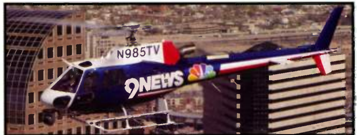
Below: When KUSA-TV launched its HD news operation in April, the station took its first step toward HD acquisition from the field with a high-definition ENG camera and microwave link mounted to its news chopper.
