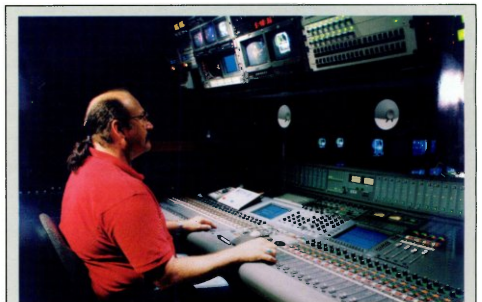
Bob Aldrige, television mixer, gets behind an AMS Neve 48-fader, 96-input Libra Live broadcast console for PBS' recent James Taylor concert broadcast. The console is part of All Mobile Video's newest all-digital audio and video truck which also features Sony gear.
