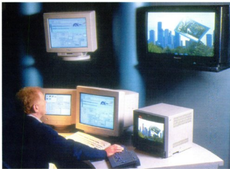
The Scitex Digital Video Sphere line of nonlinear editing systems offer compression as low as 3:1 and support for 16:9 images and QuickTime 3.0.
