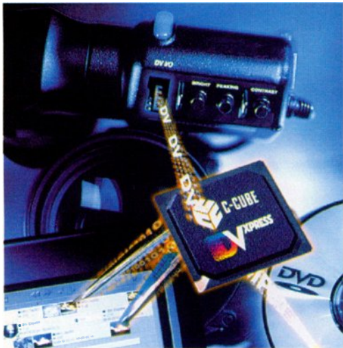
The DVXpress-MC codec from C-Cube Microsystems will transcode DV and MPEG2 compressed material.
