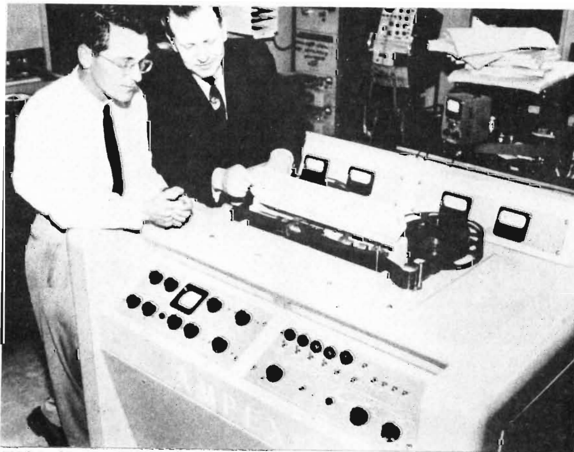
THIS is the new Ampex television tape recorder. Development of the project was in charge of Charles P. Ginsburg (l), senior project engineer in charge of video development, and Phillip L. Gundy, manager of the audio division, here inspecting the magnetic head assembly.
