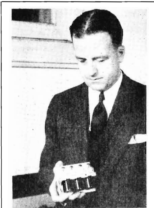
POPPELE'S LATEST —Jack Poppele, WOR chief engineer, recently elected to the board of directors as well as secretary of Bamberger Broadcasting Service, devised this midget microphone preamplifier for the Democratic convention. It weighs less than three pounds, measures less than 5 inches the longest way, has a net gain of 90 db, provides a linear response from 20 to 20,000 cycles and combines a two-circuit mixer with a three-stage, audiofrequency amplifier. It incorporates new AmerTran mid-gate audio transformers and RCA acorn tubes.
