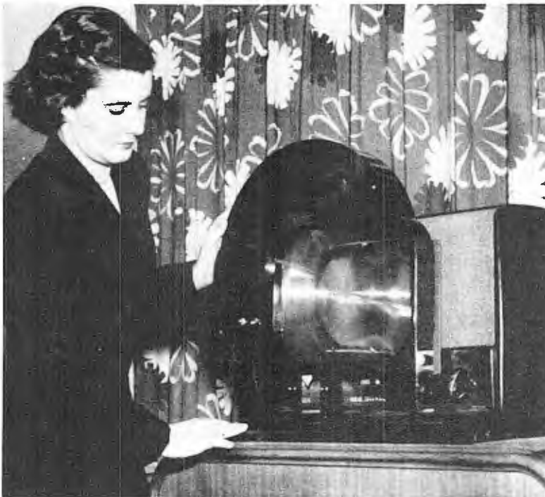
THE much discussed CBS designed and constructed color converter, which, with a simple adapter built into the set, enables a black-and-white television set also to pick up the color broadcasts of the CBS sequential color TV system, is examined by a viewer. Converter is mounted on the front of the set. When viewer wants to see color television, he merely slides it in front of his screen. If he wants to see the broadcast in black-and-white, he slides the converter aside.
