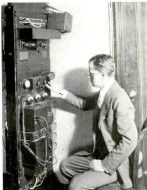
*The amplifier operator in a recording studio has ready control of the overall loudness of the record*
