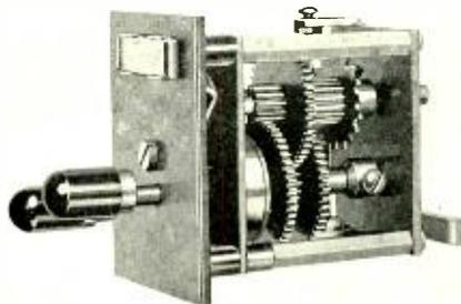
*A signalling key: turning the handle winds up a spring which drives the contact wheel*
