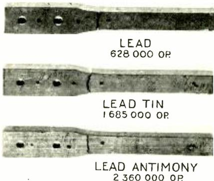
*How samples of the three cable-sheath materials failed under fatigue*
