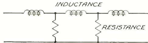
Fig. 7—Low-pass filter for filament circuits
