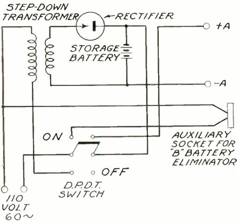
Fig. 6—Typical "trickle-charger"
