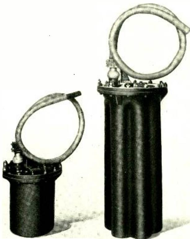
*Fig. 5—Cast-iron cases each containing 200 loading coils: left, permalloy-core coils, weight 725 pounds; right, iron-core coils, weight 1750 pounds*
