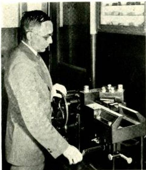
*H. A. Anderson preparing to cut a specimen of lead cable sheath on the microtome*
