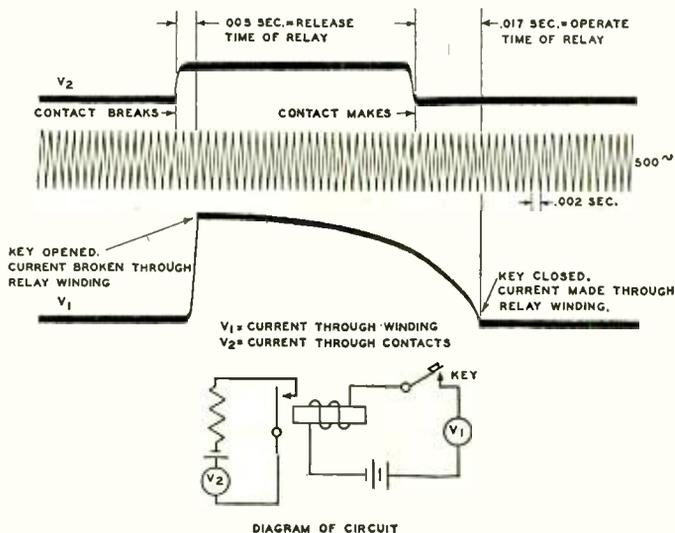
Fig. 1 — Oscillogram showing "operate" and "release" times of a relay in a typical circuit
