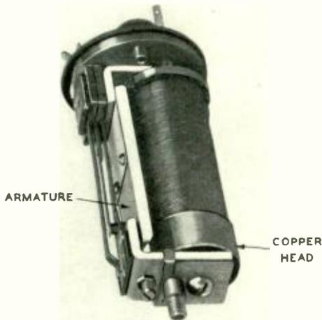
*Fig. 5 — Slow-acting relays have heavier armatures and copper heads, as may be seen in this 149-BR relay*
