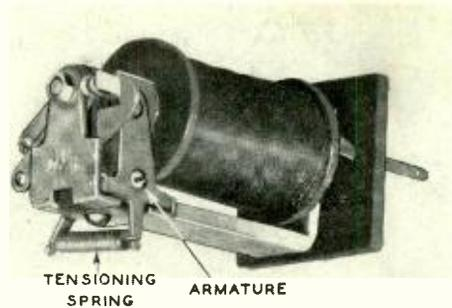
Fig. 4 — The 208 type or counting relay; one of the high-speed relays of the Bell System
