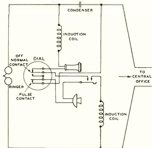
*Wiring diagram for subscriber's set showing how dialing opens the circuit*
