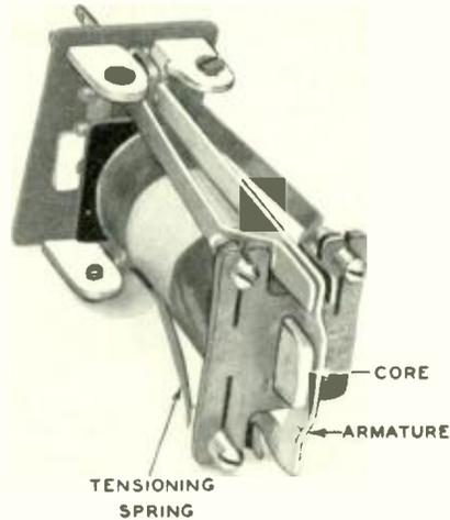
Fig. 6 — A "B" type relay used for supervisory purposes
