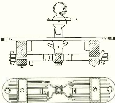
*A 51-type key, the first key lever key containing two pileups*
