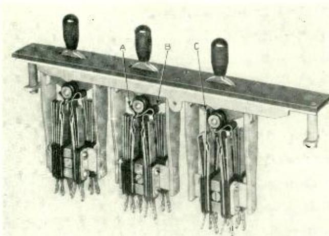
*A-1 type key, showing the mounting posts and the auxiliary frame supporting each lever unit. A, plunger spring with crimp; B, crook spring; C, straight plunger spring*
