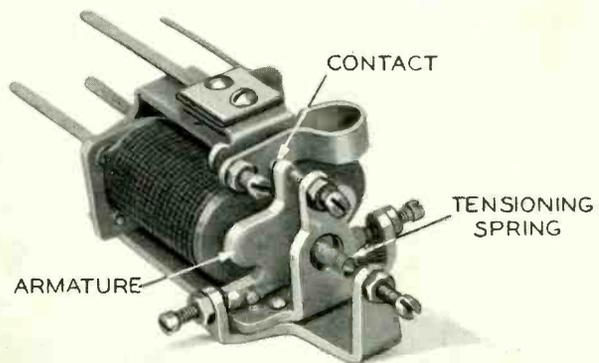
*Fig. 3 — Having, like the L type, very fast “operate” and “release” times, the stepping or 207 relay is used for but one purpose in the Bell System*
