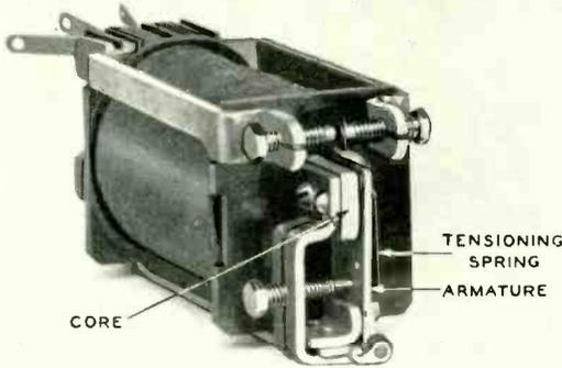
*Fig. 2 — An L type relay which finds many uses in telephone circuits where fast “operate” and “release” are required*
