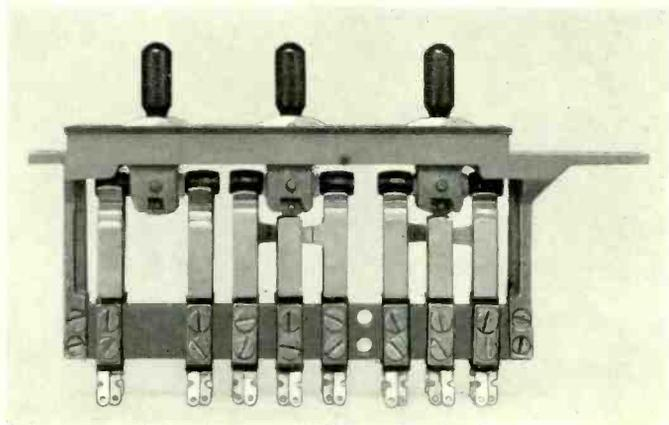
*A 463-type key, with auxiliary springs beneath two of the levers*
