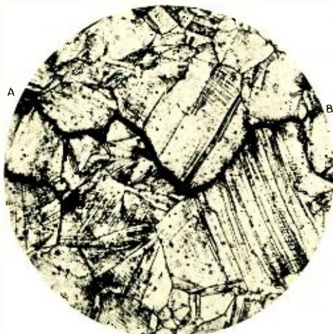
Fig. 2—In this photomicrograph of part of the wheel of Figure 1, it may be seen how the crack (AB) follows the crystal boundaries
