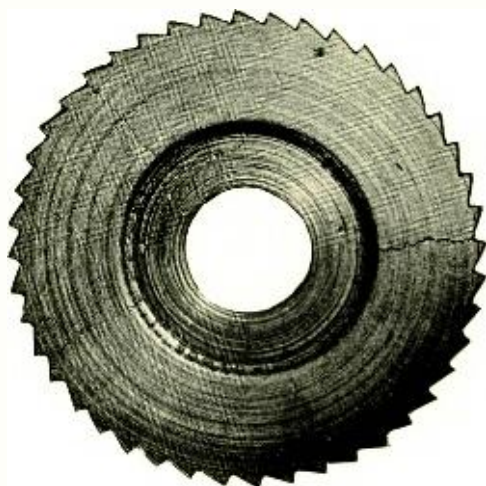
Fig. 1—The cracks in this ratchet wheel of a 200-type selector show a strong resemblance to “season cracking” of wood
