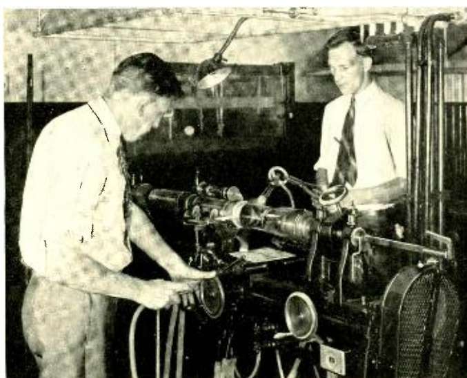
J. J. Heil and H. W. Ericsson making copper-glass seals in high-power vacuum tubes (see page 63)
