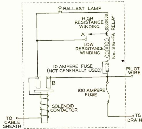
Fig. 2—Three parallel paths of different resistance are clearly indicated in this circuit diagram of the electrolysis switch
