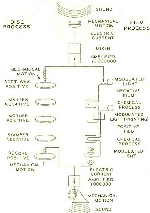
Fig. 6—Transmutations of sound from recording stage to reproducing stage
