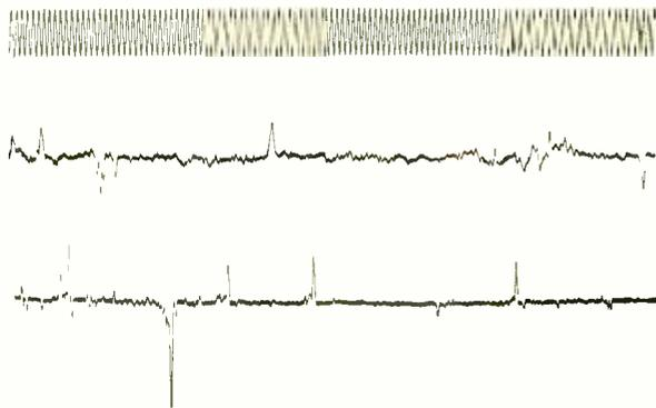
Fig. 6—Oscillograph of amplified Barkhausen effects with 1,000-cycle timing wave for comparison
