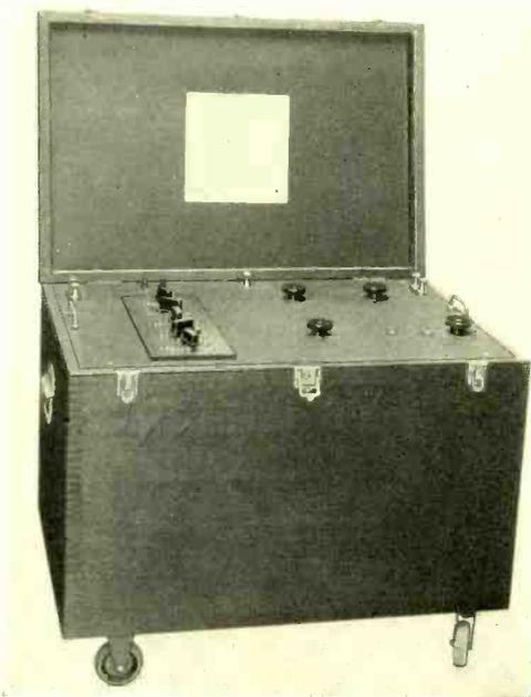
*Fig. 1—The resonance-type meter measures frequency in terms of inductances and capacitances*
