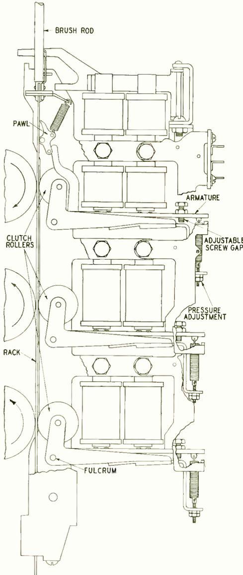
Fig. 3—A diagrammatic view of a four magnet clutch assembly shows the essential operating elements
