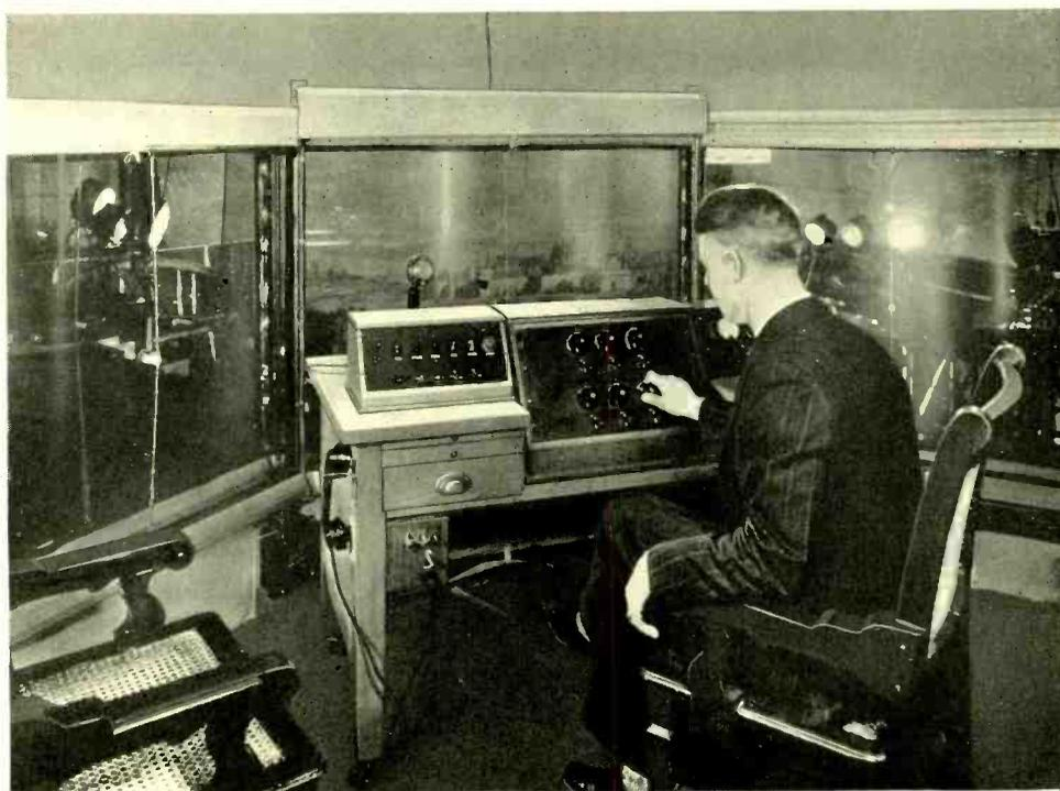
*Fig. 2—On the “mixer” table in the monitor room overlooking the stage are faders (center) for the several microphones, an overall volume indicator and volume control (right) and a communicating system (left) of lights and telephones*
