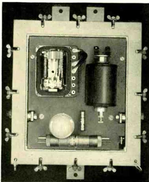
*Fig. 1—In this view of the electrolysis switch both the outer metal cases and the glass cases for the polarized relay have been removed*
