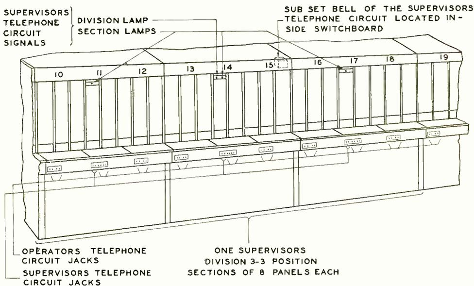
Fig. 1—Nine operator's positions form a supervisor's division and jacks are provided so that the supervisor can listen in on any operator or answer calls on her own division circuit
