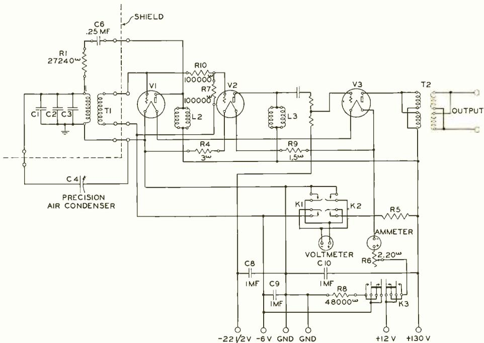
Fig. 2 — Diagram of D-85737 vacuum tube oscillator circuit
