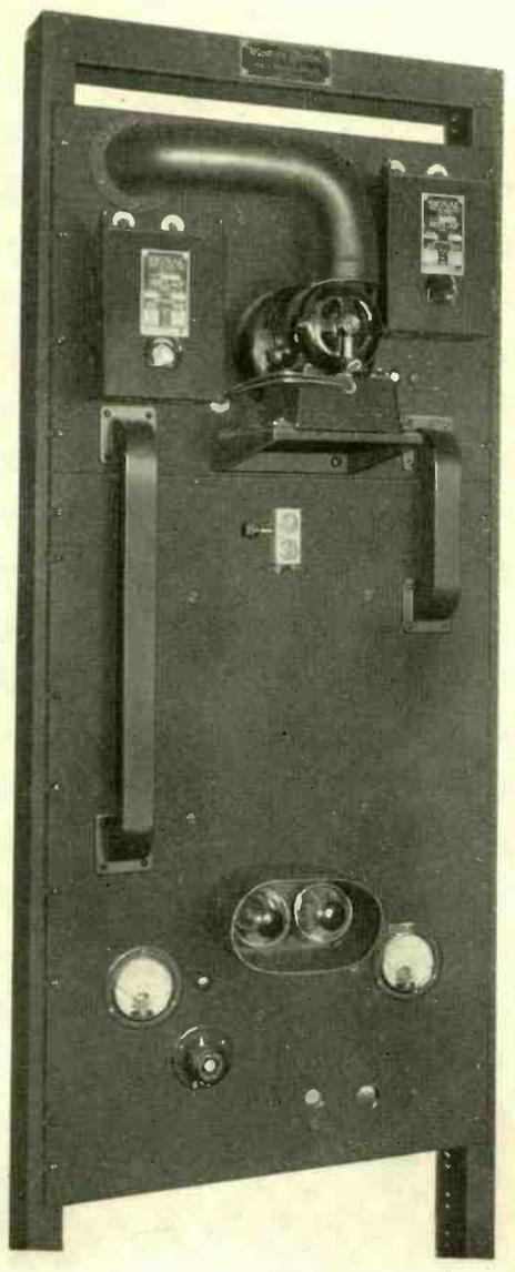
*Fig. 4—Electrically heated air is passed into the box containing the oscillator to maintain a constant temperature of about ninety-five degrees Fahrenheit*
