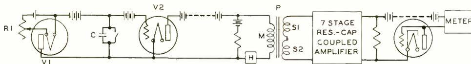
Fig. 3—Measurements of the Barkhausen effect were made by means of the circuit shown in this illustration
