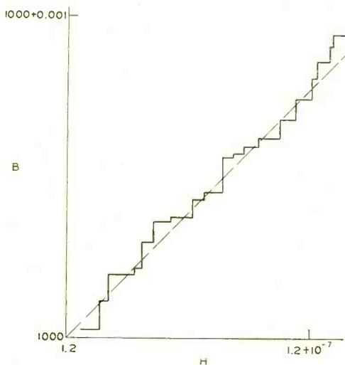
Fig. 4—The above diagram illustrates how the irregular progress of magnetization characteristic of the Barkhausen effect would appear if a small section of the magnetization curve at "T" of Fig. 2 were greatly magnified
