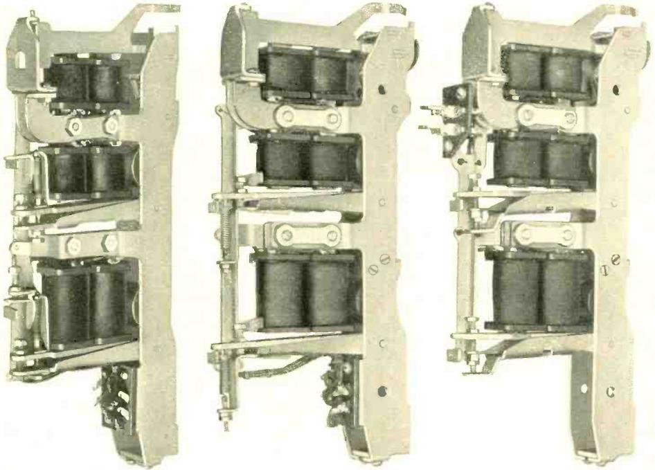
*Fig. 2 — The earliest type of clutch, shown at left, resembled those used at the present time except for the spring arrangement. The recently authorized clutch, shown at the right, differs mainly from the clutch in use at present (center) in its spring construction. A reed type spring replaces the helical spring*
