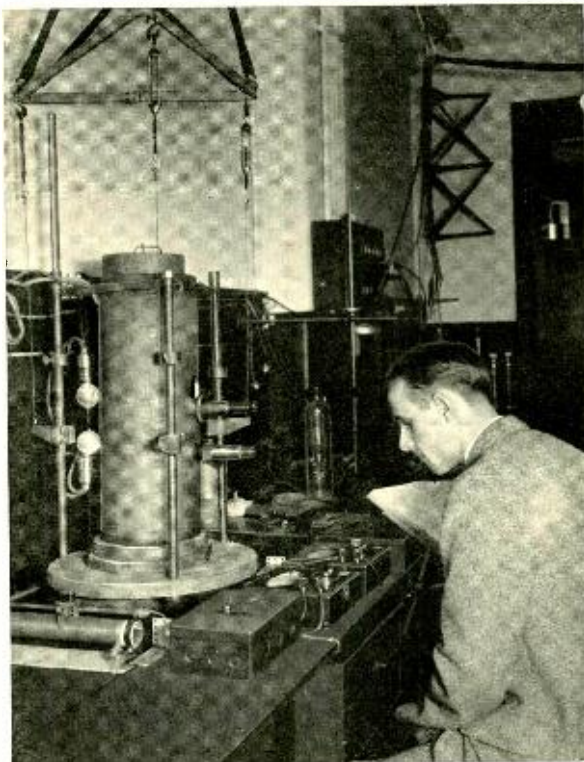
Fig. 4—C. A. Bieling with the apparatus for studying microphone action between individual granules of carbon
