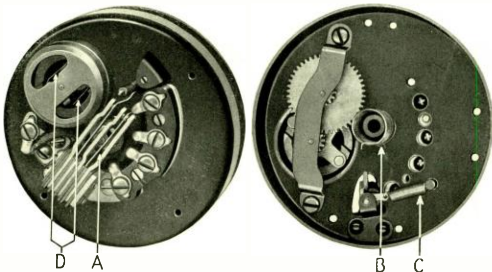
Fig. 2—Subscribers' dials contain (A) a pile-up of contact-carrying springs, helical springs for (B) motor and (C) pulsing, and (D) governor-weight springs of clock-spring steel
