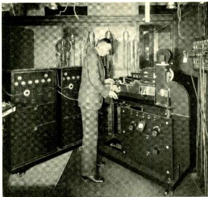
Fig. 4—I. E. Cole reading a just-developed oscillogram. The electro-magnetic unit is immediately above his left hand and the two amplifiers at his back
