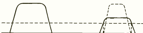
Fig. 1—Simplified diagram of signal distortion and of the action of ordinary telegraph repeaters
