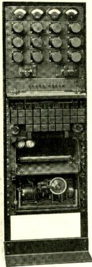
Fig. 6—A complete regenerative-repeater panel
