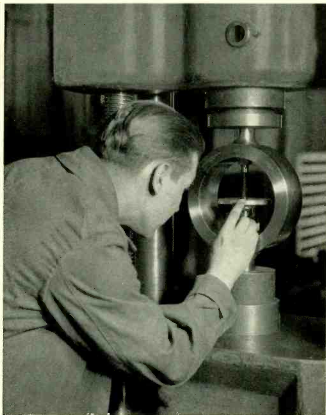
Checking the calibration of a compression testing machine in the Materials Laboratory
