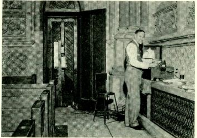
C. F. Eyring using reverberation meter for acoustic tests in St. Patrick's Cathedral
