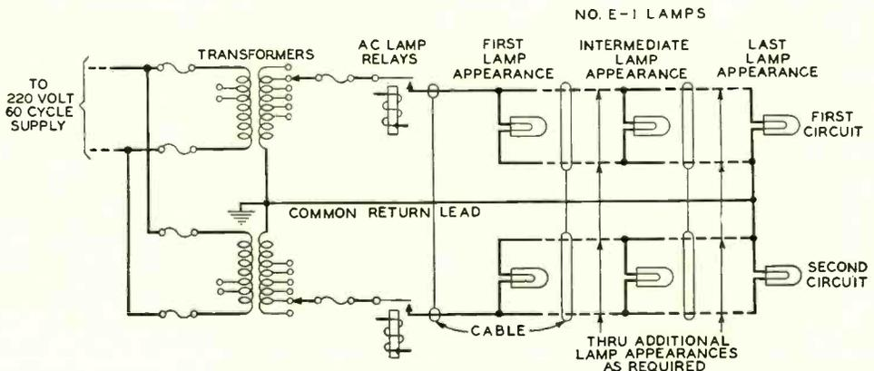
Fig. 4—Typical a-c. busy lamp multiple arrangement
