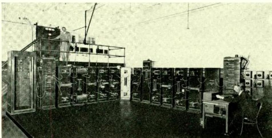
*Fig. 1—An artificial line divided into sections is mounted along two edges of an insulated platform. From the control balcony at one end there is complete control of the application of all tests*
