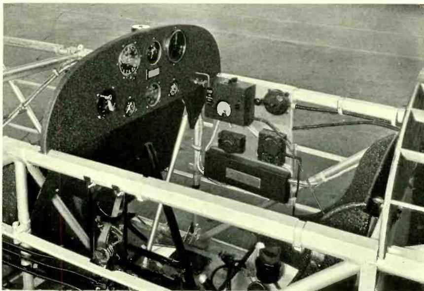
*Western Electric radio-telephone equipment for itinerant flyers installed in Fairchild airplane*
