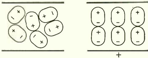
Fig. 3—A potential applied to a polar substance tends to shift its molecules from their random orientations (left) to a uniform orientation (right)
