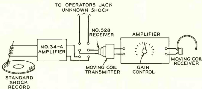
Fig. 6—Schematic diagram of acoustic-shock balance
