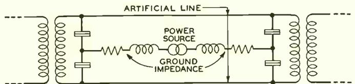
Fig. 3—Field conditions are simulated in the artificial line by inserting test potentials directly in the ground circuit
