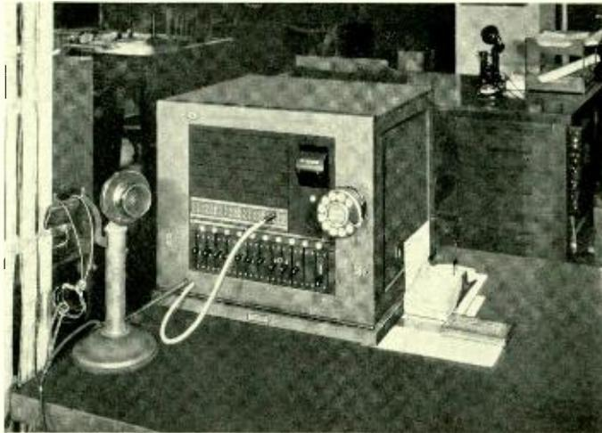
*Fig. 3—Turret for test supervisor's private desk with No. 92 jacks mounted at one side*
