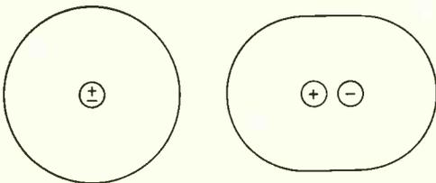
Fig. 2—In a non-polar molecule (left) the centers of opposite charge coincide; in a polar molecule (right) they do not
