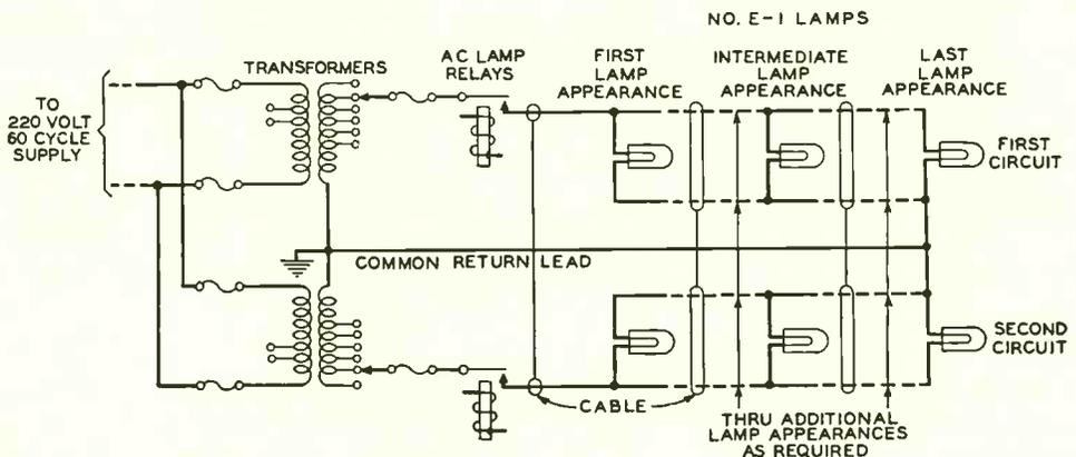
Fig. 4—Typical a-c. busy lamp multiple arrangement
