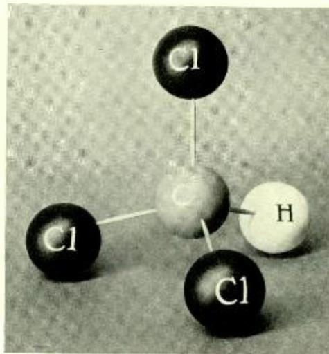
Fig. 7—Since trichloromethane (chloroform) has an asymmetrical molecule, it is a permanently polar substance
