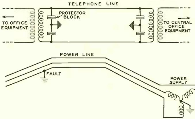
Fig. 2—Simplified schematic of one type of condition that might exist in the field
