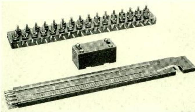
Fig. 1—Typical shellac composition parts with metal inserts embedded during the molding operation
