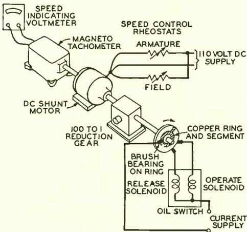
Fig. 4—Duration of disturbance is controlled by a motor-operated device which accurately times by .1 second intervals
