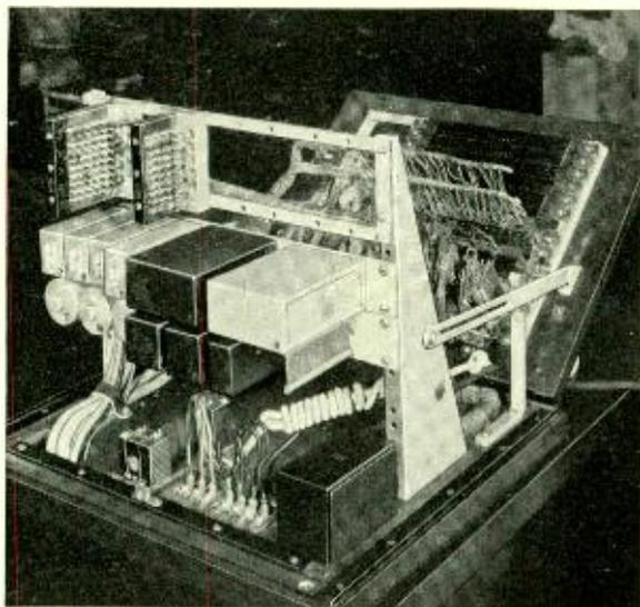
Fig. 1—The front of the new cabinet, which may be tipped forward 45 degrees, is equipped with jack fasteners on both sides of the equipment opening
