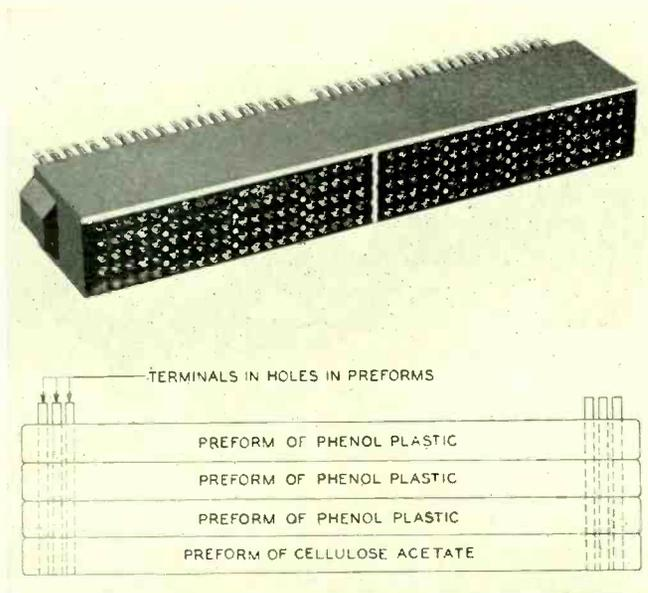
Fig. 5—The 1-C test strip, a difficult molding and engineering problem. It is now molded in one operation of phenol plastic with a veneer of cellulose acetate on the face subject to arcing
