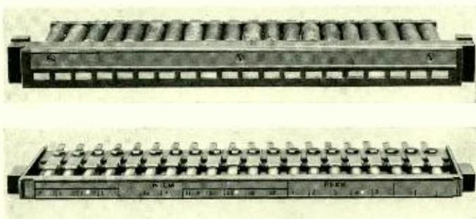
Fig. 1—(above) Until recently the common busy-indicator for toll lines has been the 42-A magnetic signal. Fig. 2—(below) In the new busy-signal strip a 1/16-inch translucent spot on the designation strip is illuminated by the newly developed E-1 lamp
