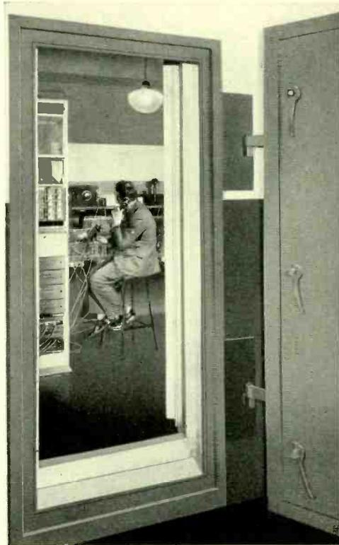
*Fig. 4—A cross talk measurement being made in one of the sound-proof rooms*
