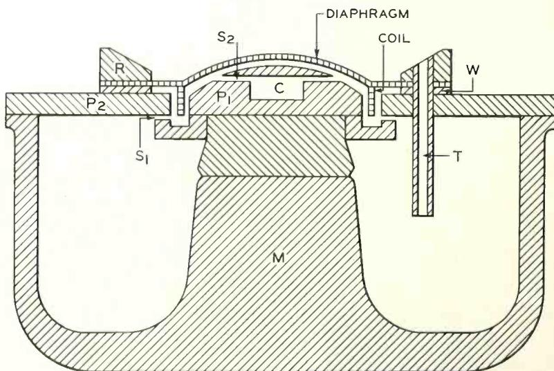
Fig. 2—A cross-section of the laboratory model shows the slit furnishing resistance control and the tube furnishing compensation for stiffness at low frequencies, as well as other features of the construction
