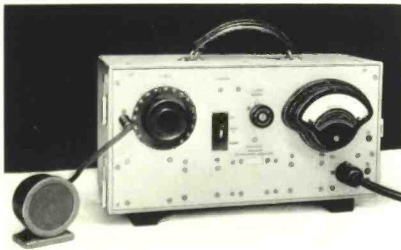
*Fig. 5—An experimental model of the new sound meter. Each of the two units weighs about 35 lbs. so that the complete unit is readily portable*
