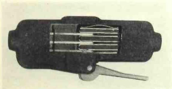
*Fig. 3—An important accessory of the new microphone is a plug and jack in which the contact pressures are high*
