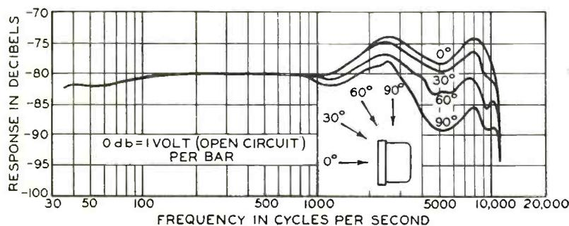
Fig. 3—Response characteristics of the commercial microphone for several angles of incidence of the actuating sound
