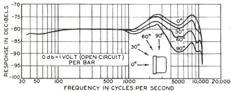
Fig. 3—Response characteristics of the commercial microphone for several angles of incidence of the actuating sound
