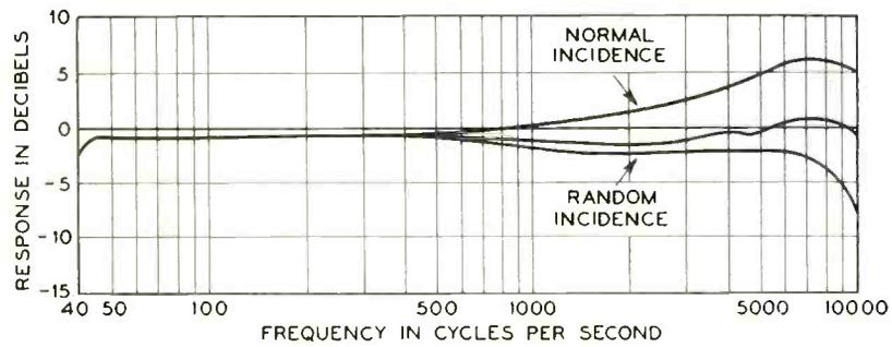
Fig. 4—The response of the microphone in actual use varies with the direction of the incident sound as indicated by the upper and lower curves of this illustration
