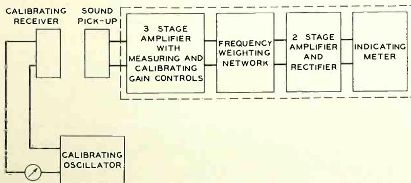
Fig. 1—An oscillator and receiver, used for calibration, form part of the equipment of the sound meter
