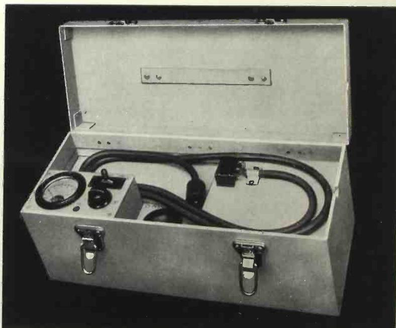
Fig. 4—The battery box includes the calibrating equipment, and has room for carrying the sound pick-up
