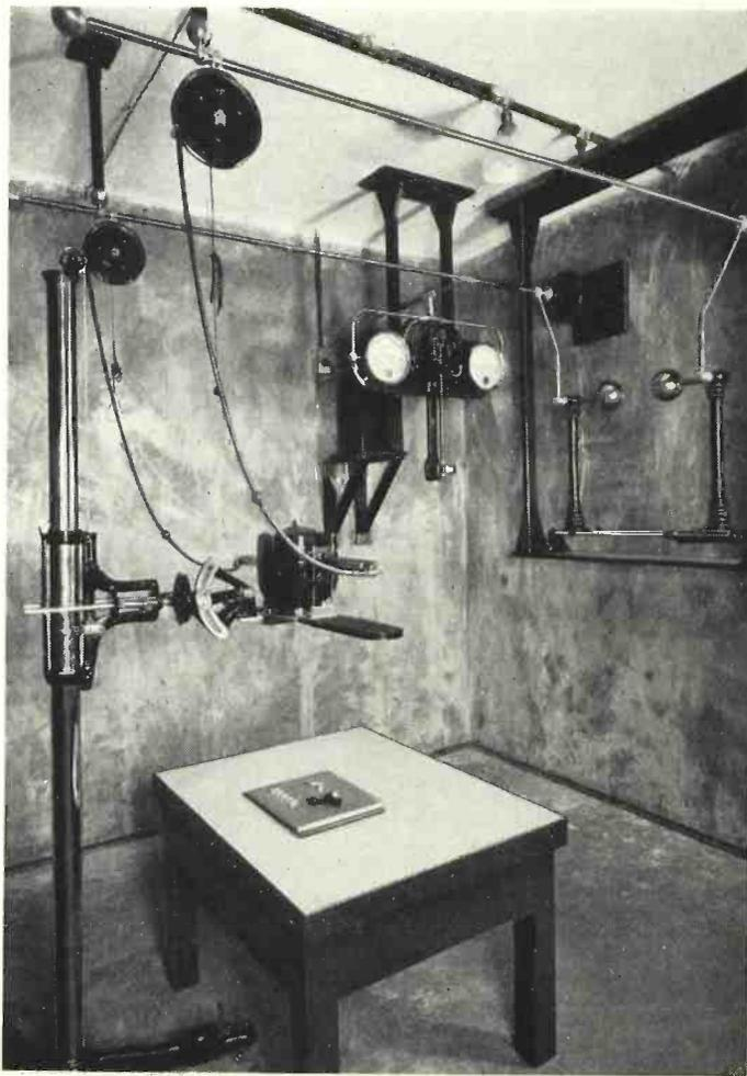
*Fig. 6—The X-ray exposure room. Parts to be X-rayed are lying on a plate holder which contains the X-ray film. The sphere gaps shown in the background are used to regulate the voltage*
