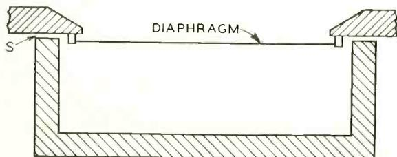
*Fig. 1—Air, moving back and forth in a narrow slit forming the only outlet of an air chamber back of the diaphragm, supplies the resistance control for the new microphone*
