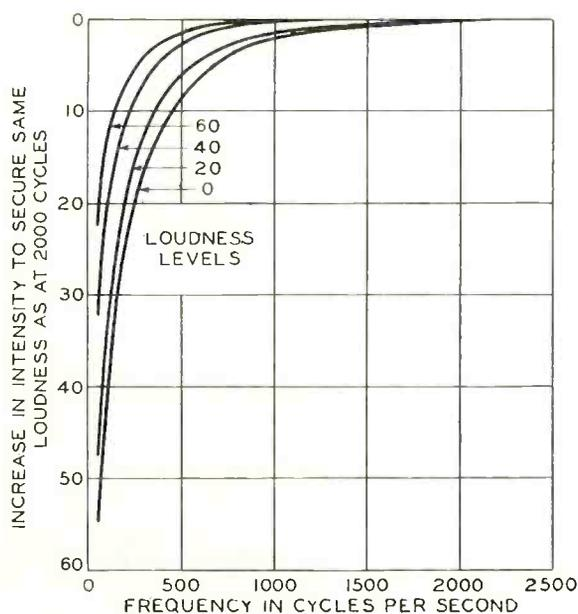
Fig. 2—To produce the same loudness, sound must be increased in pressure intensity as the frequency falls below 2,000 cycles. The relationship at four loudness levels is shown above. Levels are expressed in db
