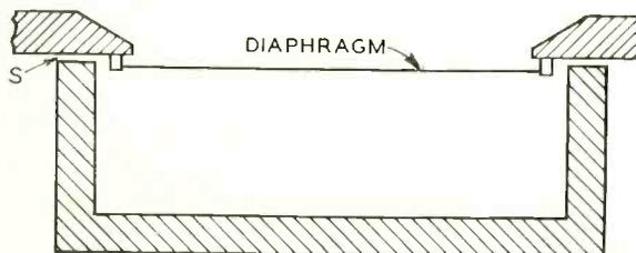
*Fig. 1—Air, moving back and forth in a narrow slit forming the only outlet of an air chamber back of the diaphragm, supplies the resistance control for the new microphone*
