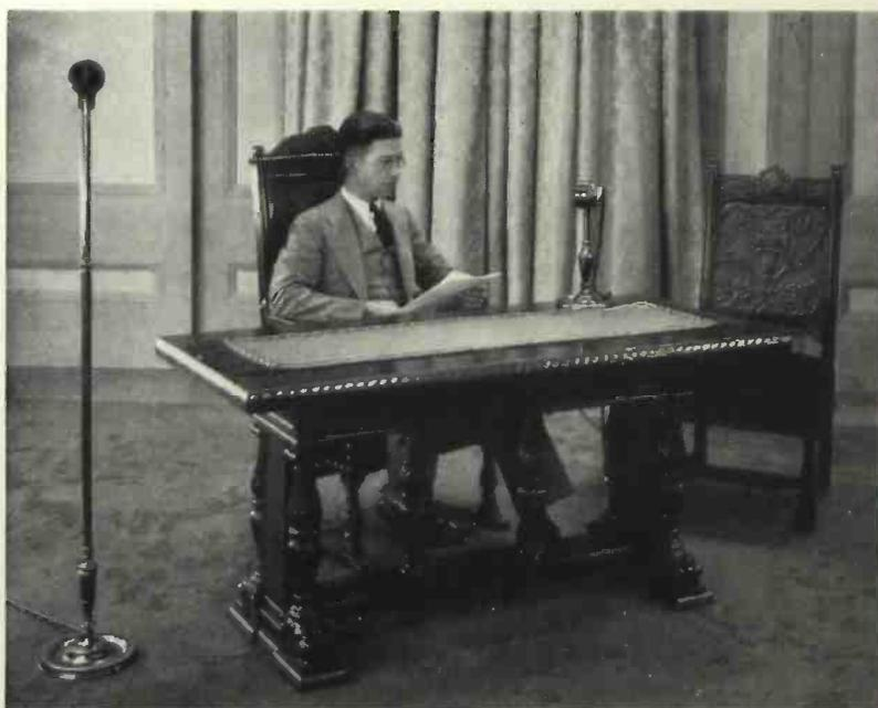
*Fig. 2—Stands have been provided for both floor and table mounting. R. L. Hanson is demonstrating the equipment in the Sound Picture Laboratory*
