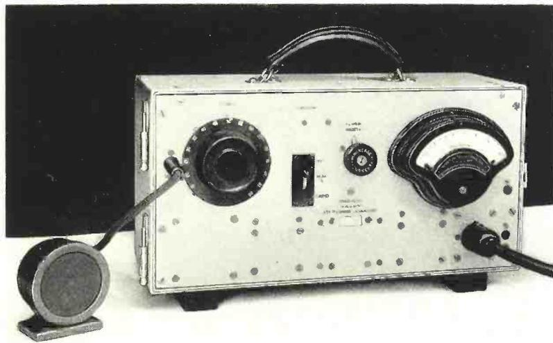
*Fig. 5—An experimental model of the new sound meter. Each of the two units weighs about 35 lbs. so that the complete unit is readily portable*
