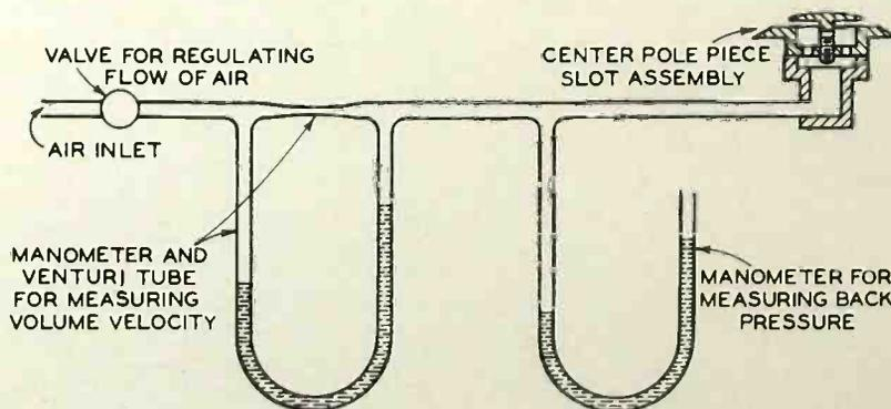
Fig. 2—By the use of such a calibrating fixture the center slot assembly can be adjusted to give the proper acoustic resistance
