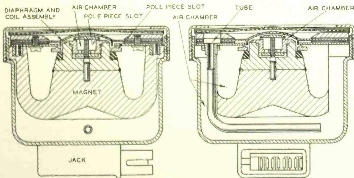
Fig. 1—Cross-sections of the commercial microphone
