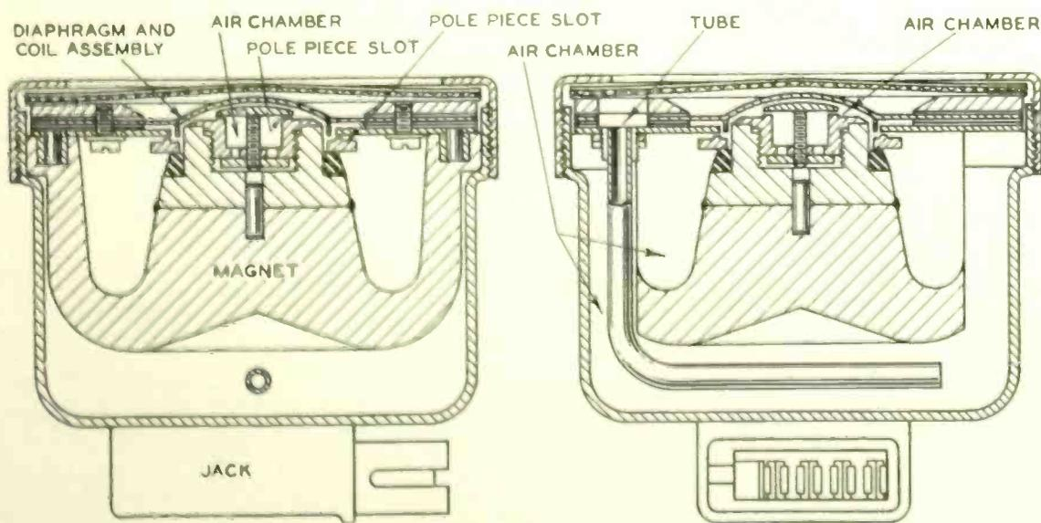
Fig. 1—Cross-sections of the commercial microphone
