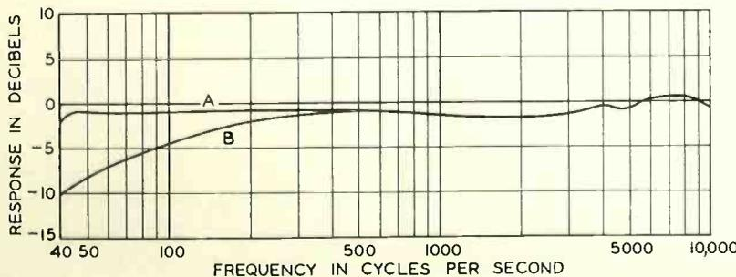
Fig. 3—The response of the complete new microphone with a constant pressure acting on the diaphragm, curve  $A$ , is practically flat from 40 to 10,000 cycles
