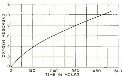
Fig. 5—The amount of oxygen absorbed by mid-continental asphalt at  $80^{\circ} C$  (expressed in cubic centimeters of oxygen per gram of asphalt) can be seen to increase with time, but at a decreasing rate
