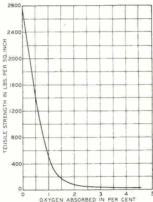
Fig. 2—The tensile strength of rubber (expressed above in pounds per square inch) decreases rapidly with increase in the amount of oxygen it absorbs (in percent of the weight of the sample)
