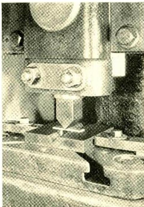
*Fig. 4—Samples of metal are formed on a punch press into 90° angles of various radii, and the smallest radius giving a satisfactory bend is determined by inspection*
