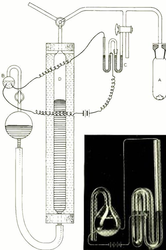
Fig. 1—The amount of oxygen absorbed by the sample in A is measured on the gas burette D. Pressure is held constant by electrolytic generation of gas from an oxalic acid solution in B, controlled by the manometer C, as shown at the lower right
