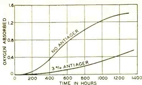
Fig. 3—A small amount of antiager will greatly decrease the amount of oxygen absorbed by rubber in a given time. The absorbed oxygen is expressed above in moles per gram-molecule of  $C_{10}H_{16}$ . The temperature of the reaction was  $80^{\circ}C$
