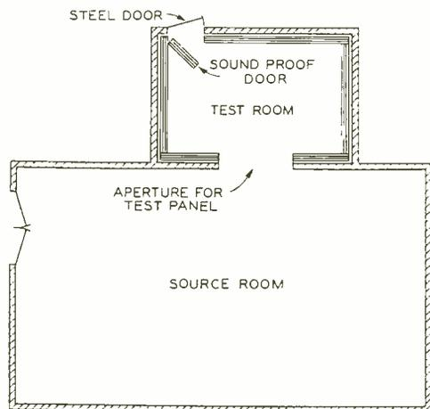
Fig. 1—Diagram of room layout for measuring the transmittivity of partitions
