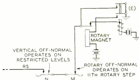
Fig. 1—Restricted service of selectors is obtained by the action of relay E when a ground appears on the RS lead
