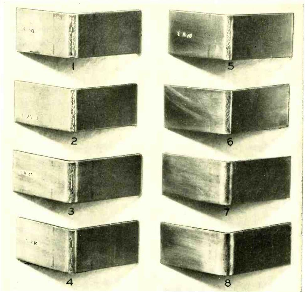
Fig. 3—Effects of bends of various radii on brass sheet
