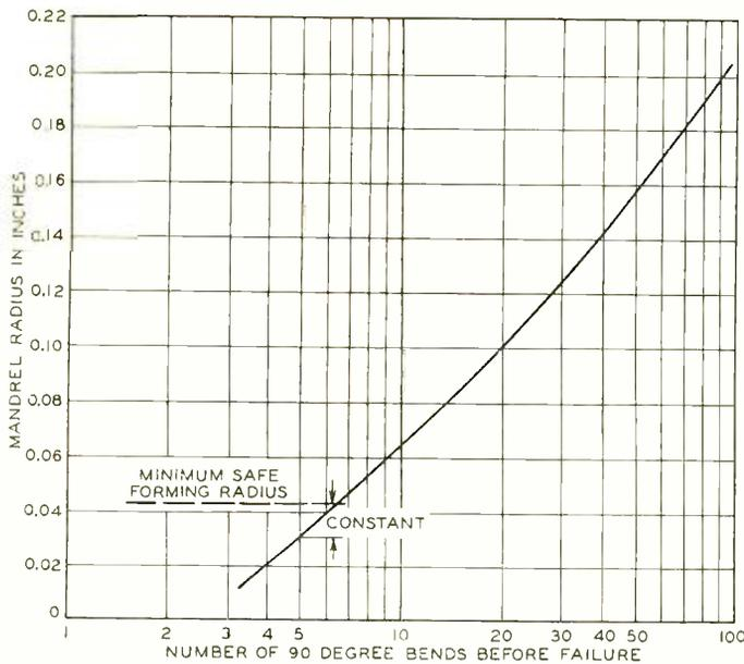
Fig. 6—Plot of radius of bend against number of bends before failure from results obtained with Amsler testing machine (24 B. & S. gauge material)
