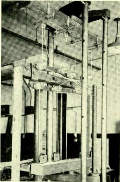
*Fig. 3—The effect of the complex load applied to transposition brackets, used where open-wire lines are transposed, is determined by reproducing the entire field installation in the testing machine*
