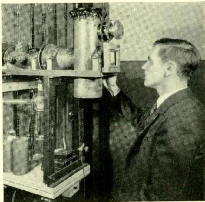
*Fig. 1—K. H. Storks of the Research Department adjusting the camera preparatory to making a photographic record of an electron diffraction pattern*
