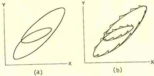
Fig. 3—The oscilloscope pattern (a) is changed to that shown at (b) when the relaxation oscillator is applied, thus indicating in this case that the oscilloscope spot is actually rotating in a clockwise direction
