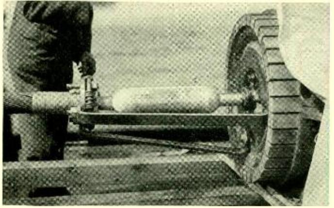
to form a water-tight housing. Nipples welded in the center of the head-plates serve as exits for the stub cables, to the sheaths of which they are soldered.
