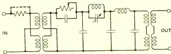
Fig. 3—Circuit schematic of frequency-weighting network for program circuit noise measurement
