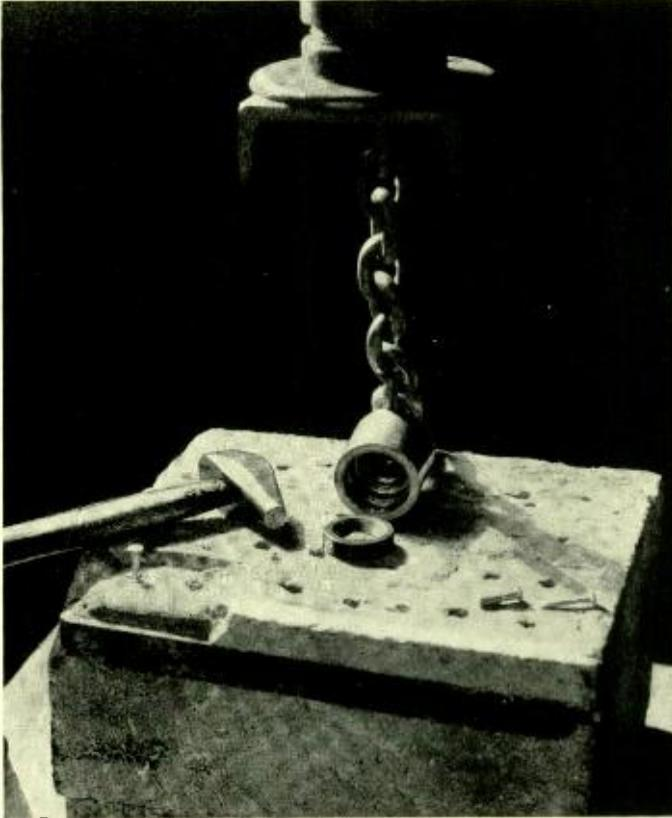
*Laboratory test for masonry anchors*
