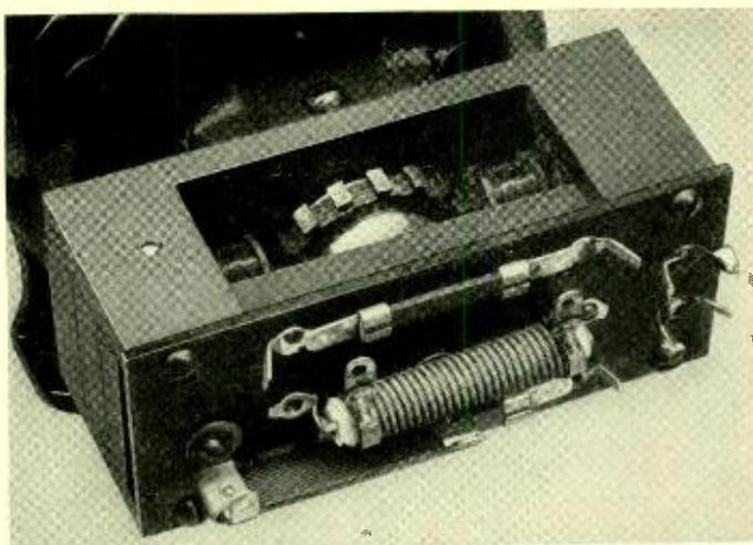
*Fig. 2—Between the inductor coils, which are mounted in a rectangular structure on the end of the inductor-alternator, is a laminated iron rotor with seventeen teeth*
