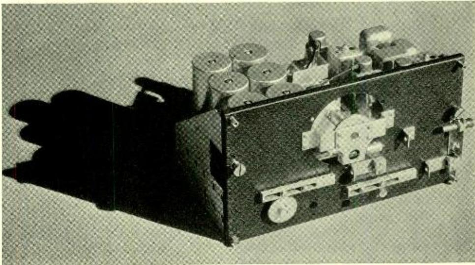
*Western Electric 20-type radio receiver developed by the Laboratories to provide a light, compact set of extreme selectivity for use in small aircraft. The receiver is designed for either remote (shown above) or local control and is provided with four frequency bands covering a range from 200 kilocycles to 10,000 kilocycles*
