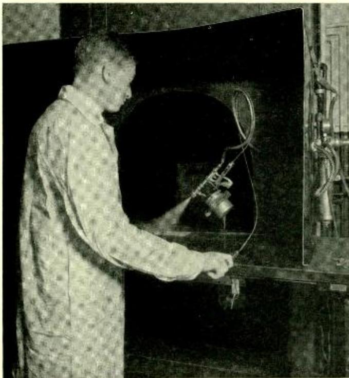
*Fig. 1—The spray gun is moved automatically at a uniform rate over the panel to be finished. H. C. Theuerer is the operator*
