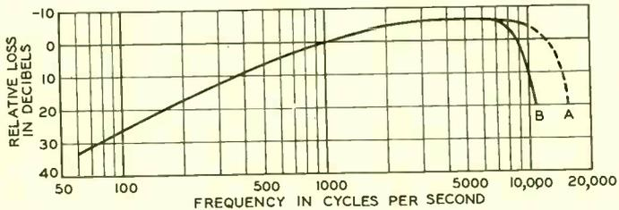
*Fig. 1—Frequency weighting curve for program circuit noise. Curve A for circuits transmitting all audible frequencies up to fifteen thousand cycles and Curve B for those cutting off at eight thousand cycles*
