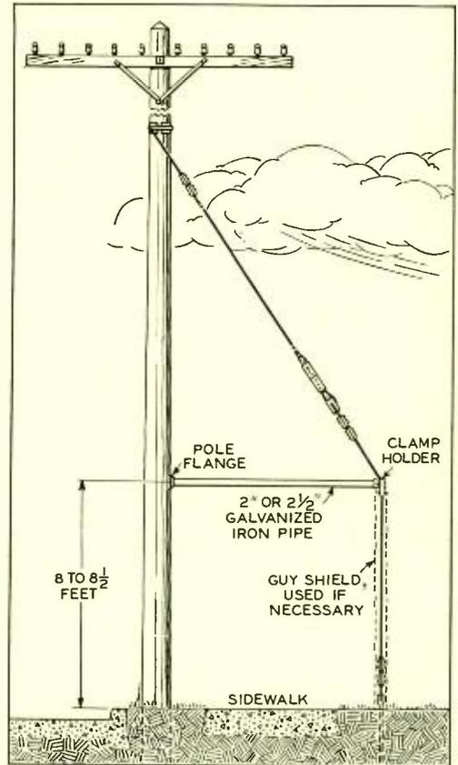
*Fig. 4—A horizontal iron pipe is used to prevent the guy strand from interfering with the right-of-way*
