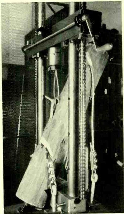
*Fig. 1—Storm guy straps used on telephone poles are tested under service load conditions by mounting them on a section of a pole held at an angle in an Amsler testing machine*
