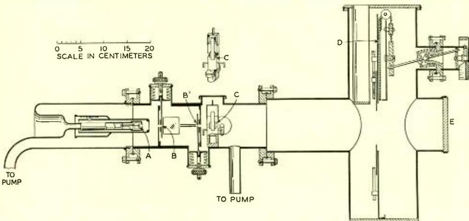
Fig. 4—Longitudinal cross-section of the electron diffraction camera
