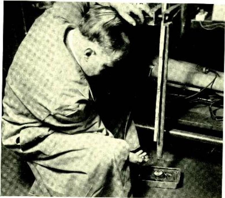
*In this impact test for goggles, W. S. Hayford is observing the effect of dropping a steel ball upon the glass from any desired height in a metal tube*
