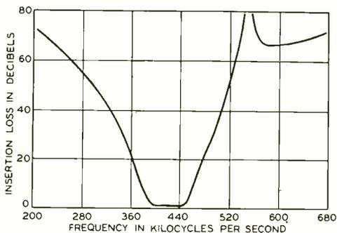
Fig. 4—Attenuation-frequency characteristic of the group filters
