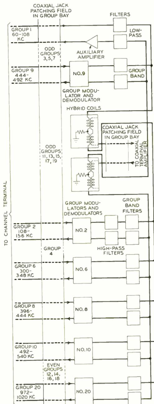
Fig. 5—Block schematic of the group terminal equipment
