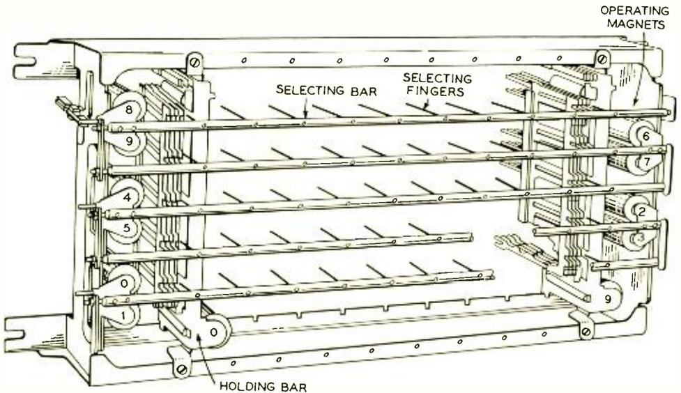
Fig. 6—Partial perspective of the crossbar switch
