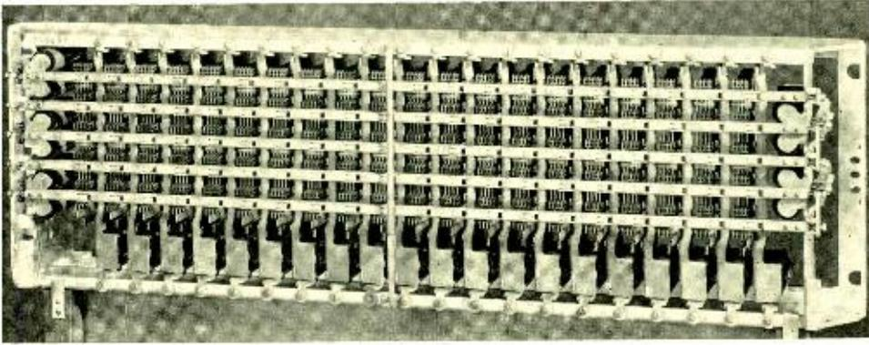
*Fig. 5—The crossbar switch has 5 selecting bars and thus 10 horizontal rows of contact groups, and up to 20 holding bars and thus 20 rows of vertical contact groups*
