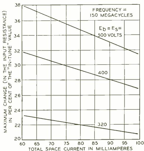
Fig. 5—Input-output reaction determined experimentally at 150 megacycles
