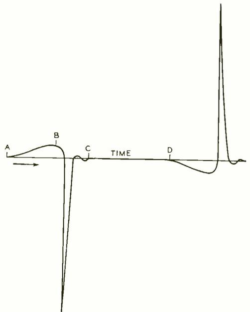
Fig. 3—Wave form of current in the output of the harmonic producer
