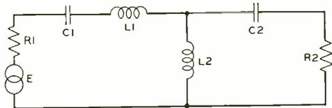
Fig. 1—Simplified schematic of the harmonic producer circuit
