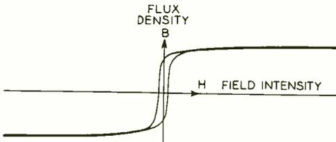
Fig. 2—Variation of magnetic flux with current in the harmonic producing coil
