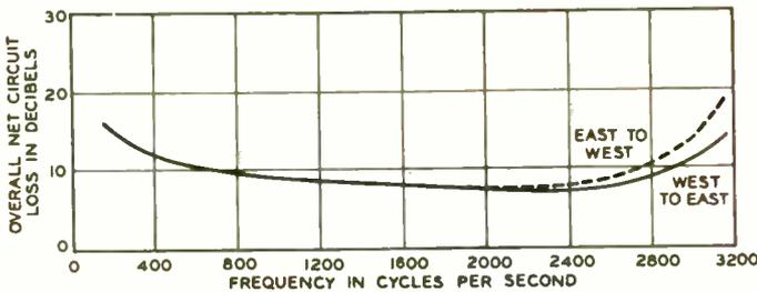
Fig. 4—Transmission characteristics of the type-H system
