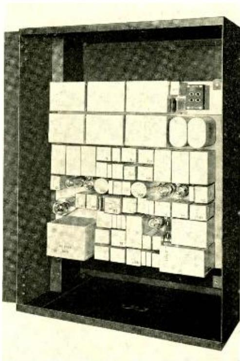
*Fig. 2—The type-H terminal may be installed either on a relay rack bay or in a metal cabinet as shown above*
