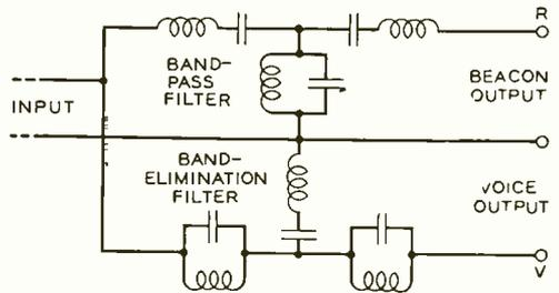
Fig. 4—Schematic of the 724A filter unit
