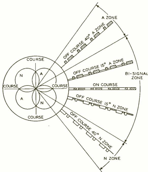
Fig. 1—Diagram of radio range system
