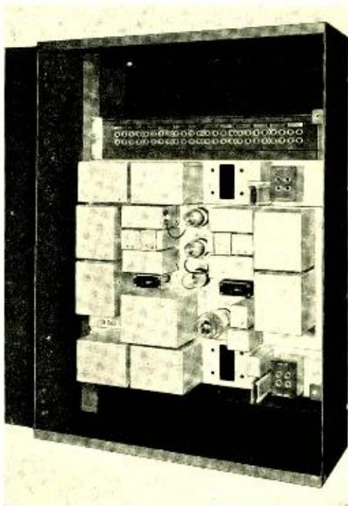
*Fig. 3—Repeater for the type-H system*
