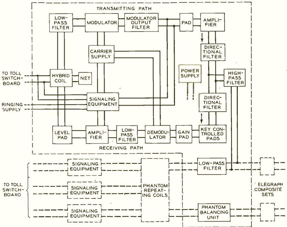
Fig. 1—Simplified block schematic of a type-H carrier terminal
