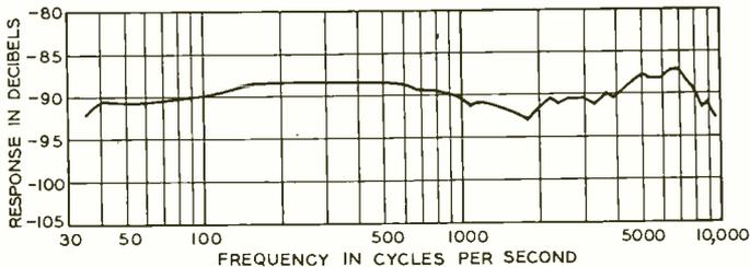
Fig. 4—Response characteristic of 633A microphone for sound at 90-degree incidence
