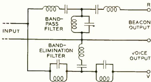
Fig. 4—Schematic of the 724A filter unit
