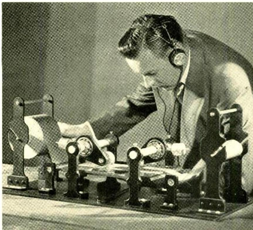
*Conducting particles are objectionable in condenser paper. In this laboratory apparatus they are detected by passing the paper between a metal roller and plate. The roller and plate terminate an electric circuit which is completed as the particle passes under the roller. The particles are counted by an electric recorder or by listening to the clicks in a telephone headset. W. J. Kiernan is shown operating the apparatus*
