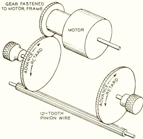
Fig. 5—Gear arrangement for the adjusting drive
