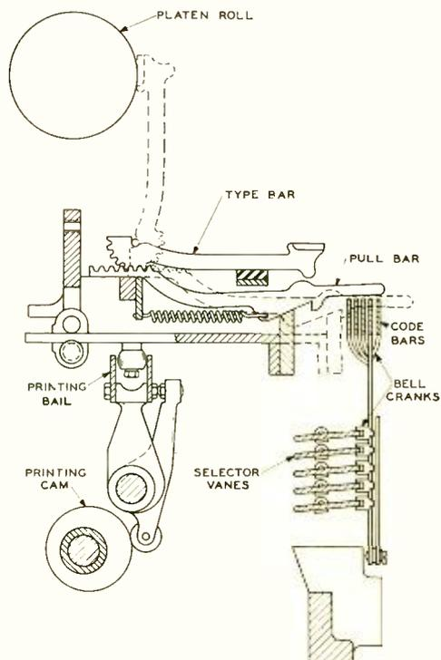
*Fig. 4—Printing action of the 15-type teletypewriter. When the code bars have been positioned by a code signal one of the pull bars drops into a line-up of slots in the code bars. A projection on the pull bar then catches the lever connected to the printing bail as it advances. This raises the type bar and prints the character*
