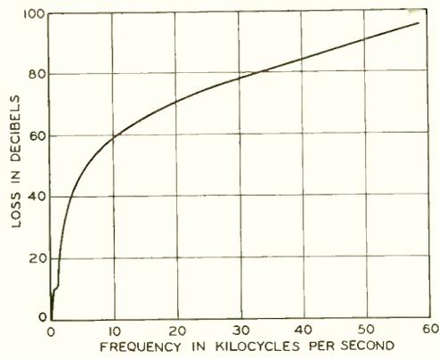
Fig. 3—Longitudinal insertion loss characteristic of a typical filter as measured between fixed resistances
