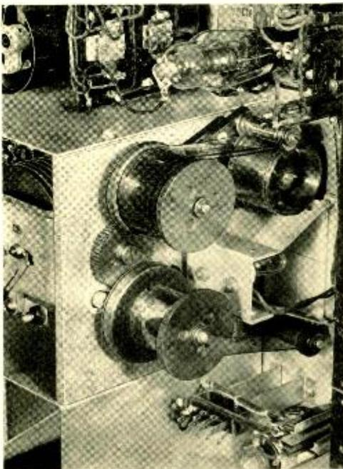
*Fig. 3—Film and sprocket arrangement for the 17B oscillator scale*
