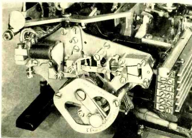
Fig. 1—Holding magnet and selector mechanism of the 15-type teletypewriter
