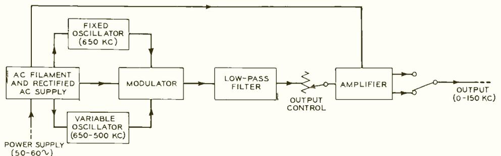
Fig. 1—Block schematic for the 17B oscillator
