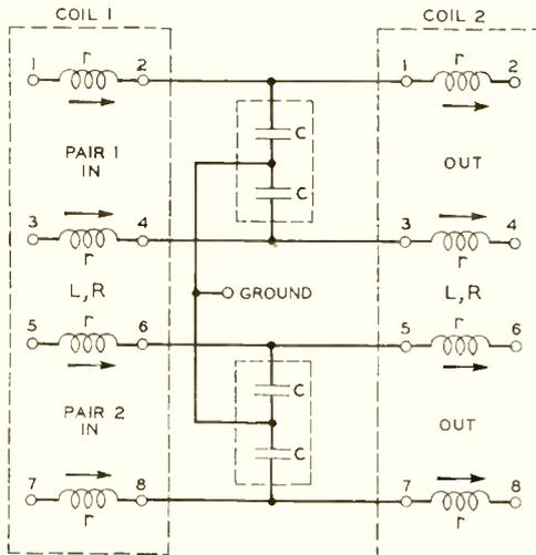
Fig. 1—Schematic diagram of the 81A noise filter
