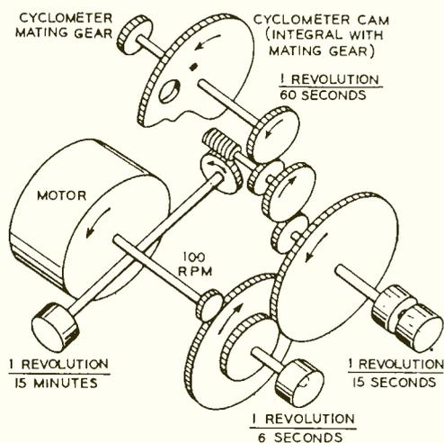
Fig. 3—Gear arrangement used to drive the various commutators
