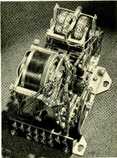
*Fig. 1—Time unit with cover removed showing the four timing commutators*
