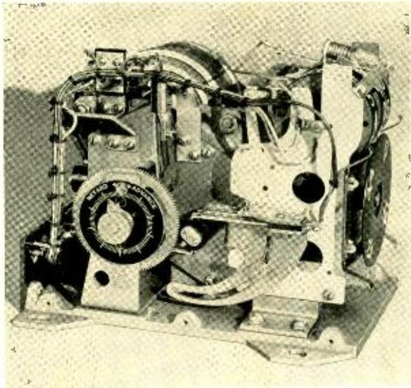
*Fig. 2—Side view of time unit showing moveable bracket, at the lower right, for adjusting the duration of the announcing period*
