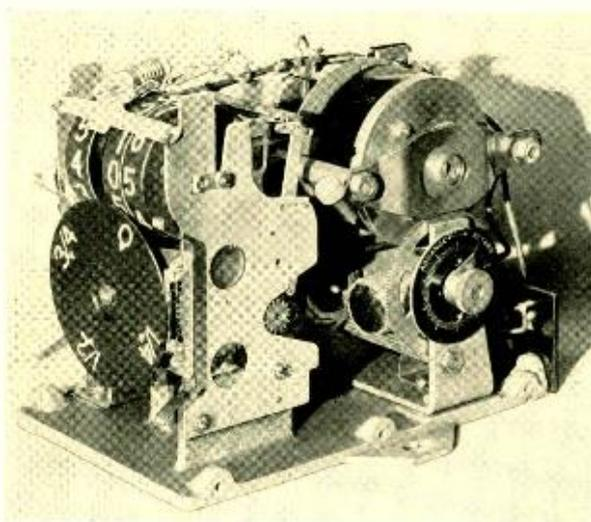
Fig. 4—View of time unit showing cyclometer, at the left, and the adjusting knob and gears for rotating the motor winding, at the right
