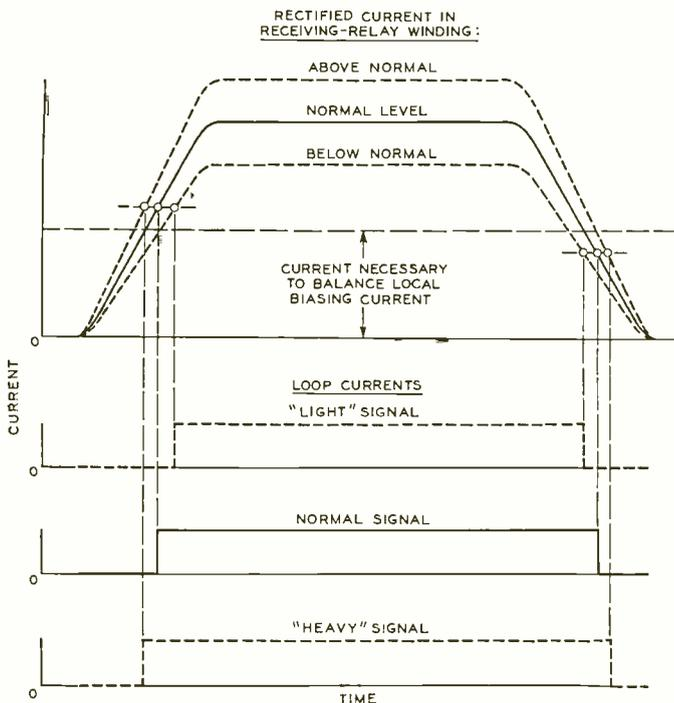
Fig. 1—Telegraph signals of various levels, shown on the upper line, result in received signals of different lengths
