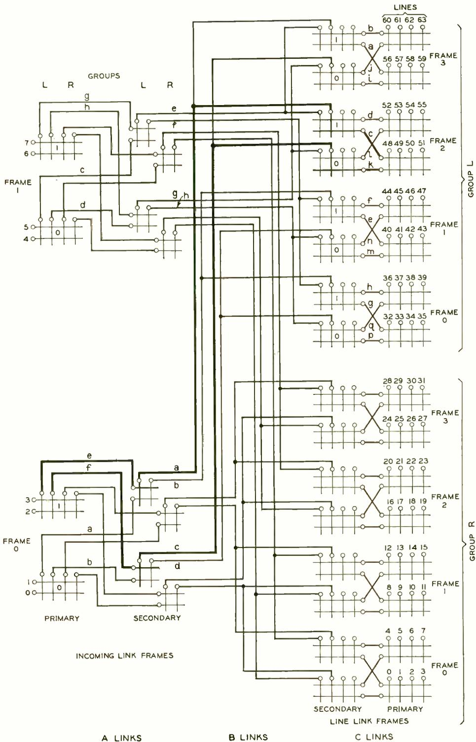
side of the incoming primary switches run to the left side of the incoming secondary switches. The arrangement of the links can be illustrated by considering, for example, a call from trunk 3 to line 48. The two possible A links will be *e* and *f*; the B links will be *a* and *c*; while the C links will be *c* and *k*.
