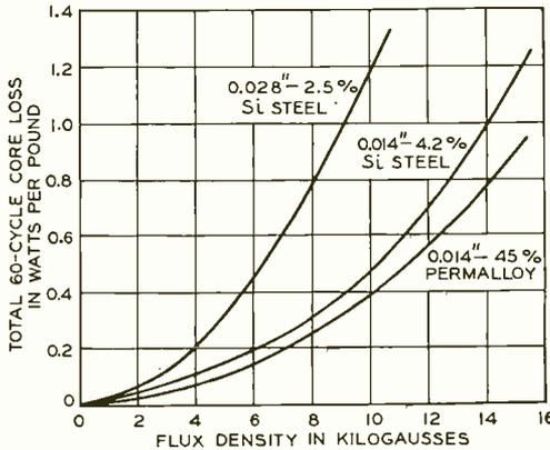
Fig. 4—Core losses in typical materials determined with an Epstein testing set
