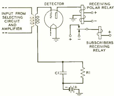
Fig. 2—Schematic of level compensator
