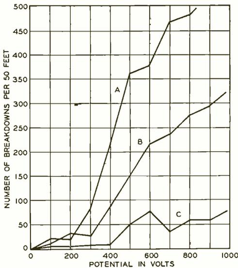
Fig. 3—Thick enamel showed fewer defective places than thin. Thickness—A, .0004 inch; B, .0006 inch; C, .0008 inch
