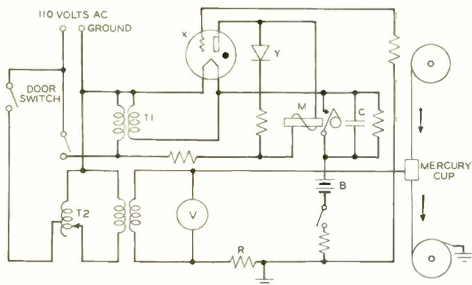
Fig. 1—When the insulation on the wire breaks down at the mercury cup the grid potential of the thyatron tube changes to make it conduct and operate the register M
