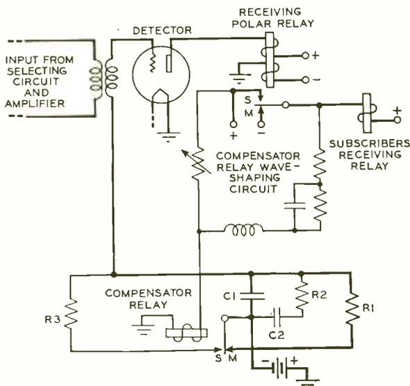
Fig. 3—Complete diagram of level compensator
