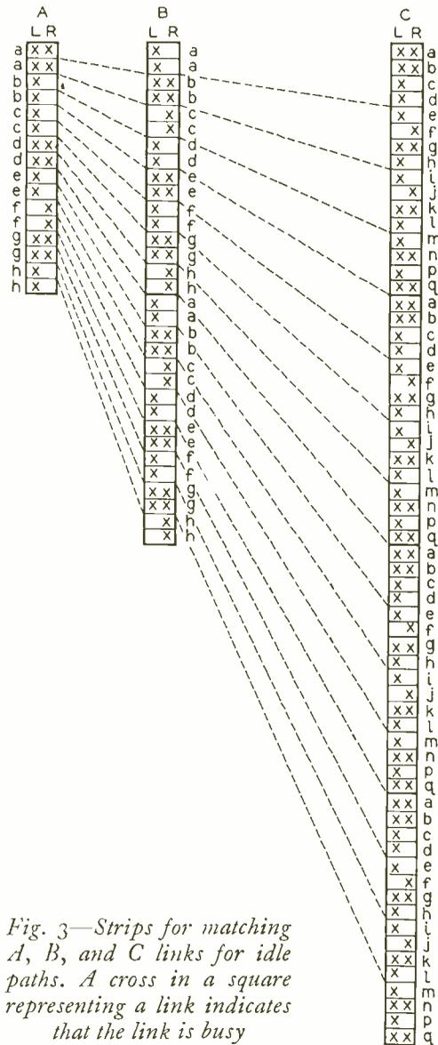
Fig. 3—Strips for matching A, B, and C links for idle paths. A cross in a square representing a link indicates that the link is busy
