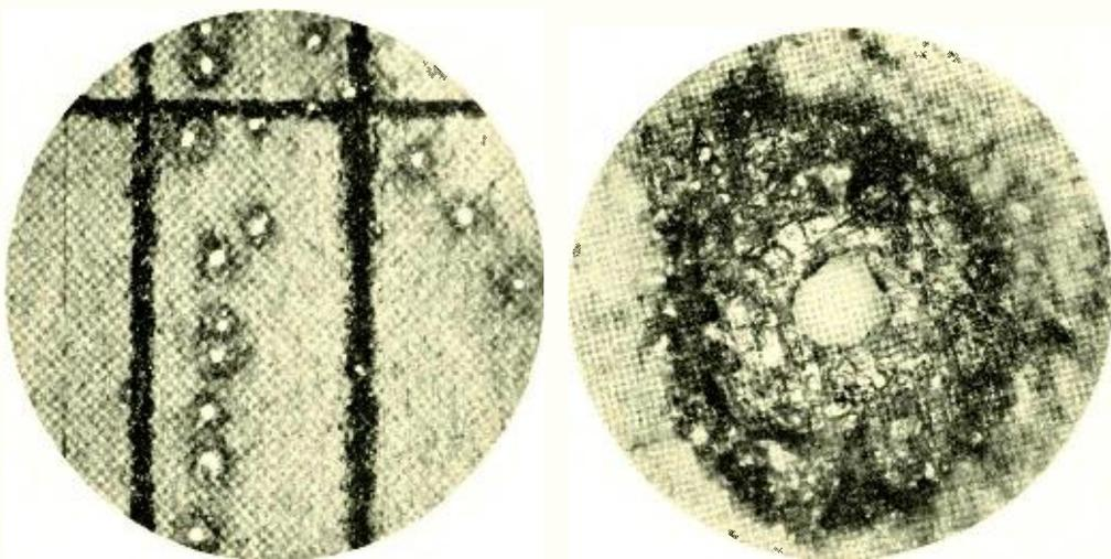
*Fig. 3—Photomicrographs of spark records which show the perforations in the chart and the dark rings where the wax was melted by the spark. The divisions on the chart represent hundredths of a second*
