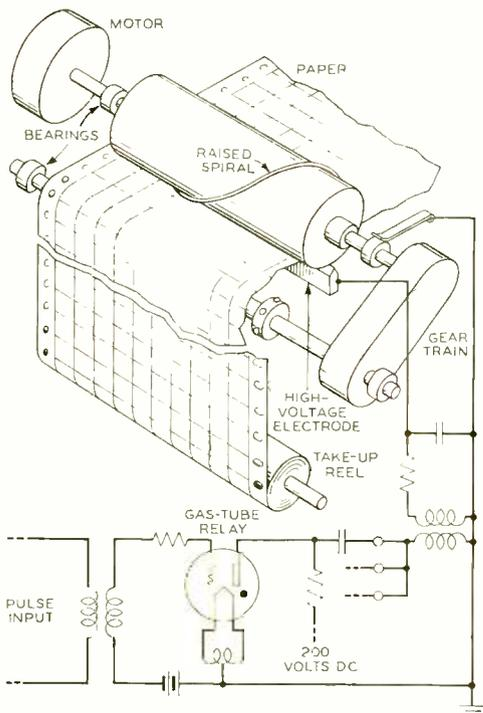
Fig. 1—A metal drum with a spiral raised above its surface rotates above a moving sheet of recording paper which passes over a long knife-edged electrode. Sparks from the knife edge to the spiral perforate the paper at points which depend on the angular position of the rotating drum
