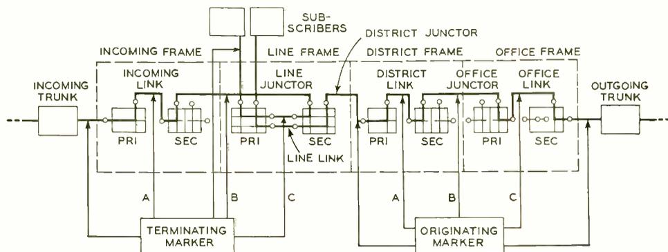
Fig. 1—Block schematic of crossbar system showing ABC trunking scheme
