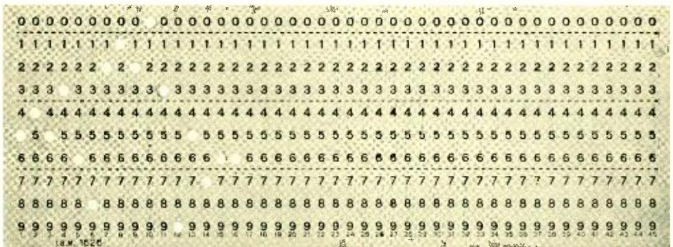
Fig. 4—One of the types of cards used for recording the sixteen-digit numbers used to represent each call. The number represented by this card is 4,829,330,312,066,466
