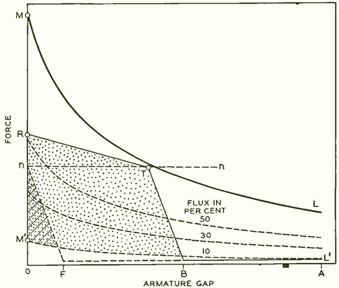
Fig. 5—Force-displacement designed for original clutch with a series of curves to show decreasing magnetic force
