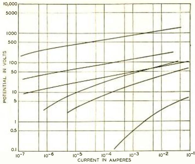
Fig. 5—An indication of the variety of characteristics which can be obtained in silicon carbide varistors
