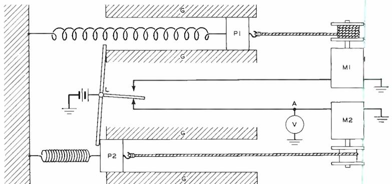
Fig. 2—A multivibrator when represented mechanically becomes more complicated than an oscillator because two moving elements are required, each drawn one way by a spring and the other by a motor, and the surfaces they slide on offer resistance to motion
