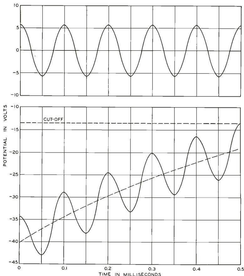
Fig. 7—An indication of how an oscillator voltage, upper diagram, superimposed on voltage  $e$ —dashed curve—results in a voltage, lower solid line, that reaches the cut-off value at a period that is a multiple of the oscillator period
