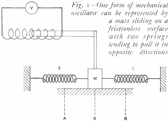
Fig. 1—One form of mechanical oscillator can be represented by a mass sliding on a frictionless surface with two springs tending to pull it in opposite directions
