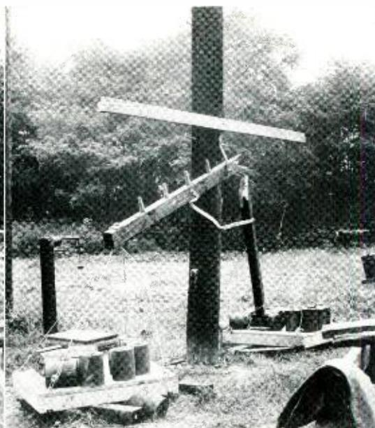
*The short break in the crossarm shown above is characteristic of jack pine. Long breaks, illustrated in the headpiece, occur in Douglas fir*
