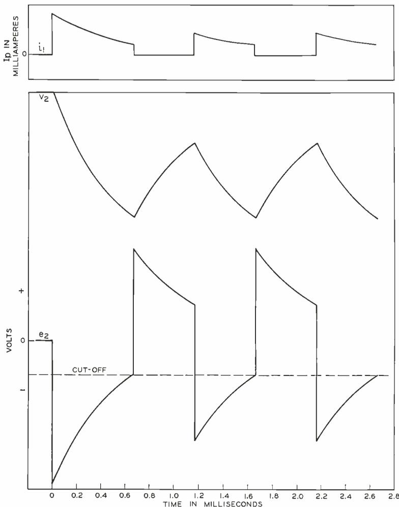
Fig. 4—The voltage  $V_2$  across  $C_2$  of Figure 3, and the corresponding voltage  $e_2$  across  $R_{g2}$  as time progresses. The upper diagram shows the plate current of tube 1 over the same interval
