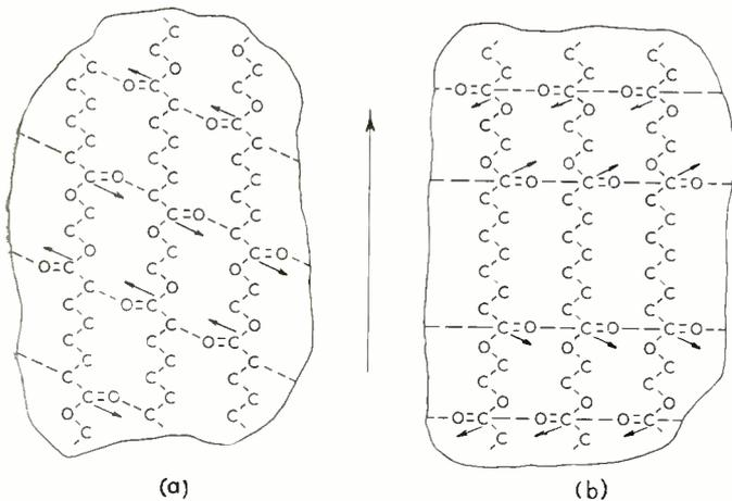
Fig. 4—Schematic of polyethylene sebacate (a) and polyethylene azelate (b) molecules. The former has an even number of atoms between the C=O groups which permits stronger association with adjacent molecular layers and is therefore the stronger plastic
