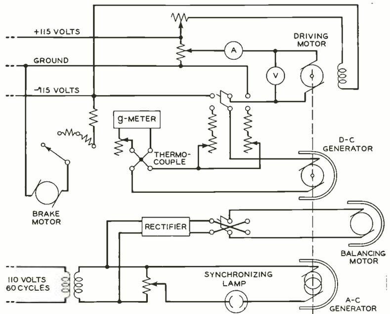
Fig. 1—Simplified circuit diagram for the 1,000-g centrifuge
