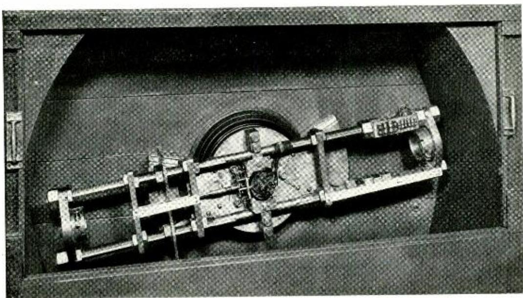
**I**N ITS more usual form, a centrifuge is employed to separate materials of different specific gravities by the action of centrifugal force. At high rotational speeds, objects tend to be driven radially outward with an acceleration proportional to the square of velocity. Heavy particles in a rotated liquid, for example, may be separated from the liquid by this action, or on a mixture of liquids, the heavier may be separated from the lighter. The actual ac-
