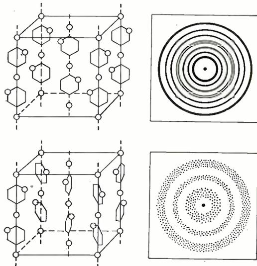
Fig. 5—Ordered (upper) and disordered (lower) cellulose chain molecules with the X-ray diagram of each. Sharp lines are obtained with an ordered specimen
