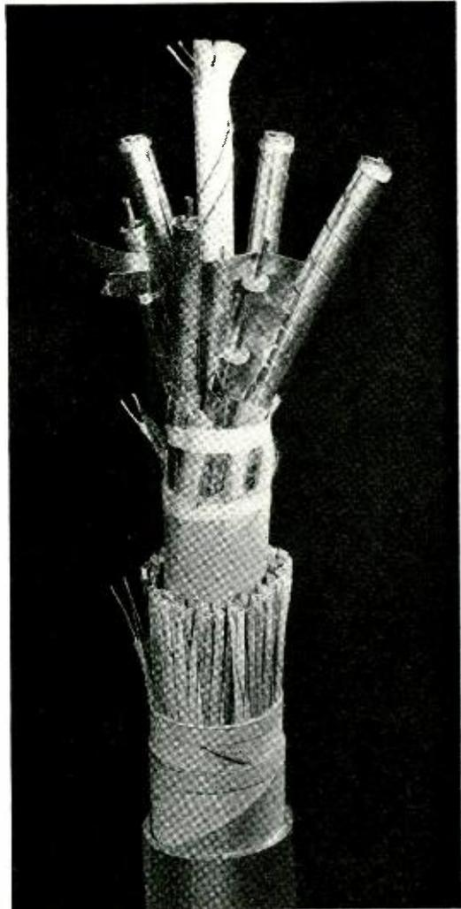
*Coaxial cable now being installed between Terre Haute and St. Louis. It consists of 6 coaxial conductors, 21 quads and several service pairs*
