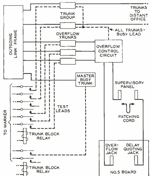
Fig. 1—Simplified schematic of connections to overflow circuit
