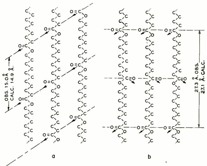
Fig. 3—Schematic of polyundecanoate (a) and polydecanoate (b) molecules showing the difference in frequency of occurrence and position of the active C=O groups which determine the strength of attraction between adjacent molecular layers and hence the strength of the plastic
