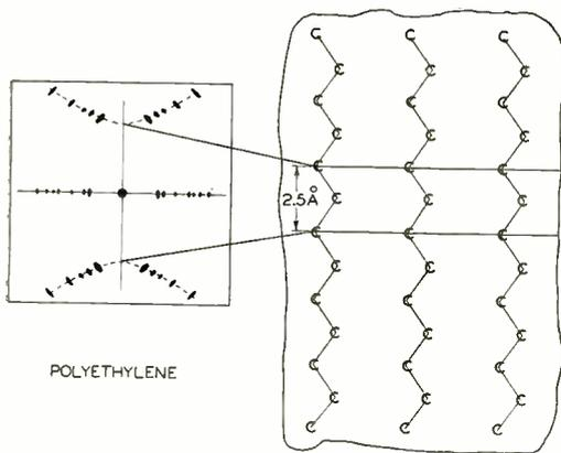
Fig. 2—Chain structure of the polyethylene molecule showing the location of the atoms which produce its X-ray pattern
