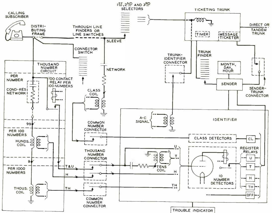
Fig. 1—Identifier circuit for the automatic ticketing system in Culver City, California
