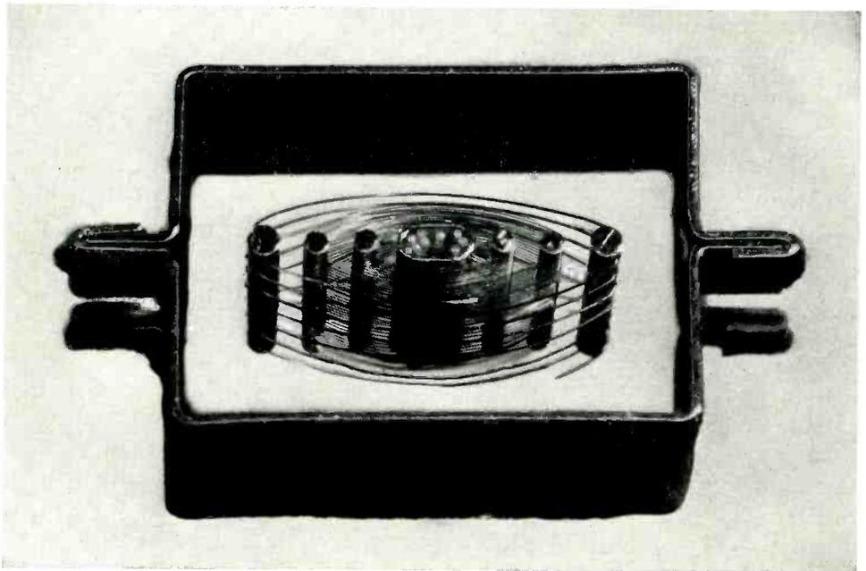
*Fig. 2—A cross-section of the 6AK5, shown about ten times actual size, reveals the small size and close spacing of the elements that have made it possible to secure the desired characteristics*
