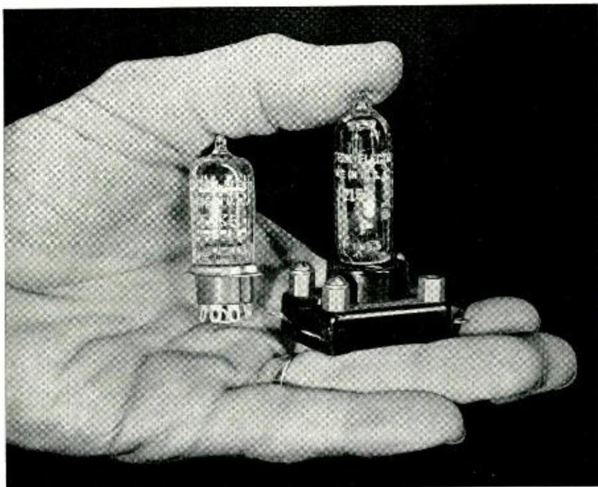
Fig. 3—The 6AK5 tube (left) is distinctly smaller than the 215A peanut tube developed during World War I and has approximately twelve times the transconductance. Their characteristics follow:
