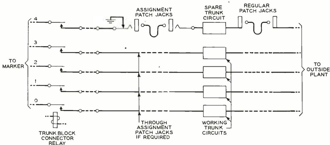
Fig. 4—Block schematic of arrangements for assignment patching
