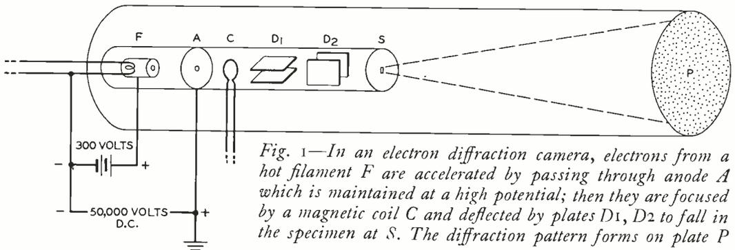
Fig. 1—In an electron diffraction camera, electrons from a hot filament *F* are accelerated by passing through anode *A* which is maintained at a high potential; then they are focused by a magnetic coil *C* and deflected by plates *D*<sub>1</sub>, *D*<sub>2</sub> to fall in the specimen at *S*. The diffraction pattern forms on plate *P*
