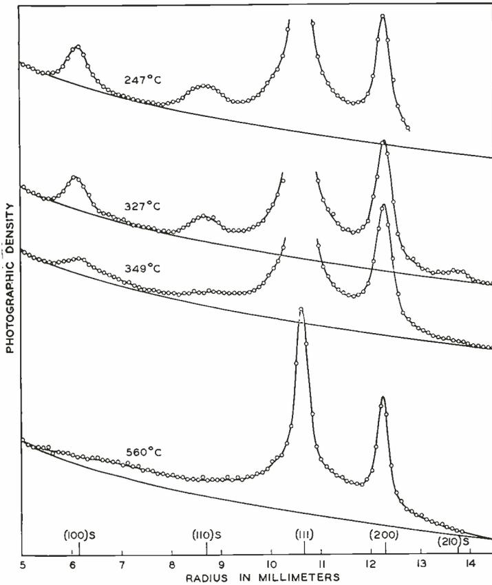
Fig. 8—Microphotometer curves show the gradual change from sharp rings to diffuse bands when an ordered film is heated. Up to 327 degrees C. there is no marked difference in the shape of the peaks but at 349 degrees considerable broadening has occurred
