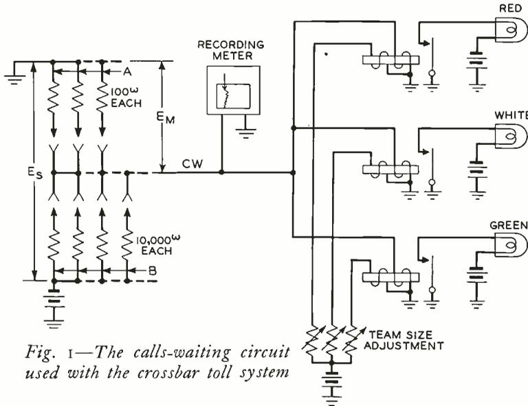
Fig. 1—The calls-waiting circuit used with the crossbar toll system
