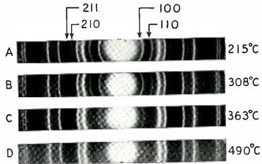
Fig. 9—Diffraction patterns from  $\text{Cu}_3\text{Au}$  films heated to different temperatures in the electric furnace. Patterns A and B have the diffuse bands which indicate that the imperfect ordering had not been appreciably affected by heating to 300 degrees C. In patterns C and D, taken at higher temperatures, broadening of these bands shows that ordering had decreased
