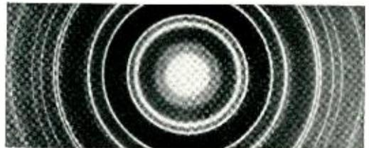
Fig. 2 (left)—Diffraction pattern from an unordered film of  $\text{Cu}_3\text{Au}$  alloy before heat treatment
