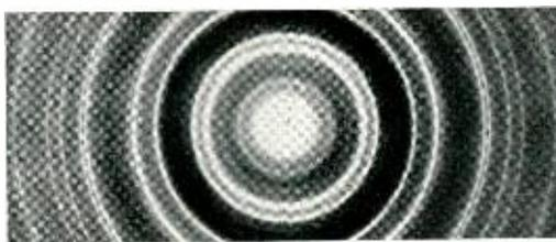
Fig. 5—Diffraction pattern of a  $Cu_3Au$  alloy film after it had been heated for sixteen hours at 194 degrees C. The two diffuse rings next to the central spot indicate that annealing had caused partial ordering of the atoms
