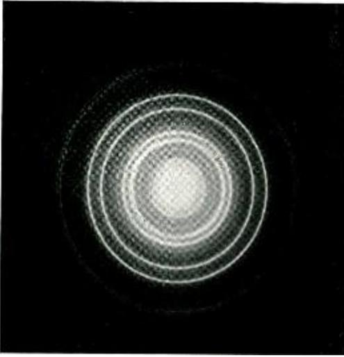
Fig. 6—Atoms of  $Cu_3Au$  alloy become completely ordered when heated for sixteen hours at 270 degrees C. This is shown by the two sharp rings next to the central spot
