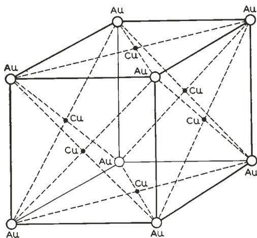
Fig. 4—Face-centered cubic structure, showing the position of the gold and copper atoms in the alloy crystals when ordered. The gold atoms are at the corners of the cube and those of copper in the center of the faces
