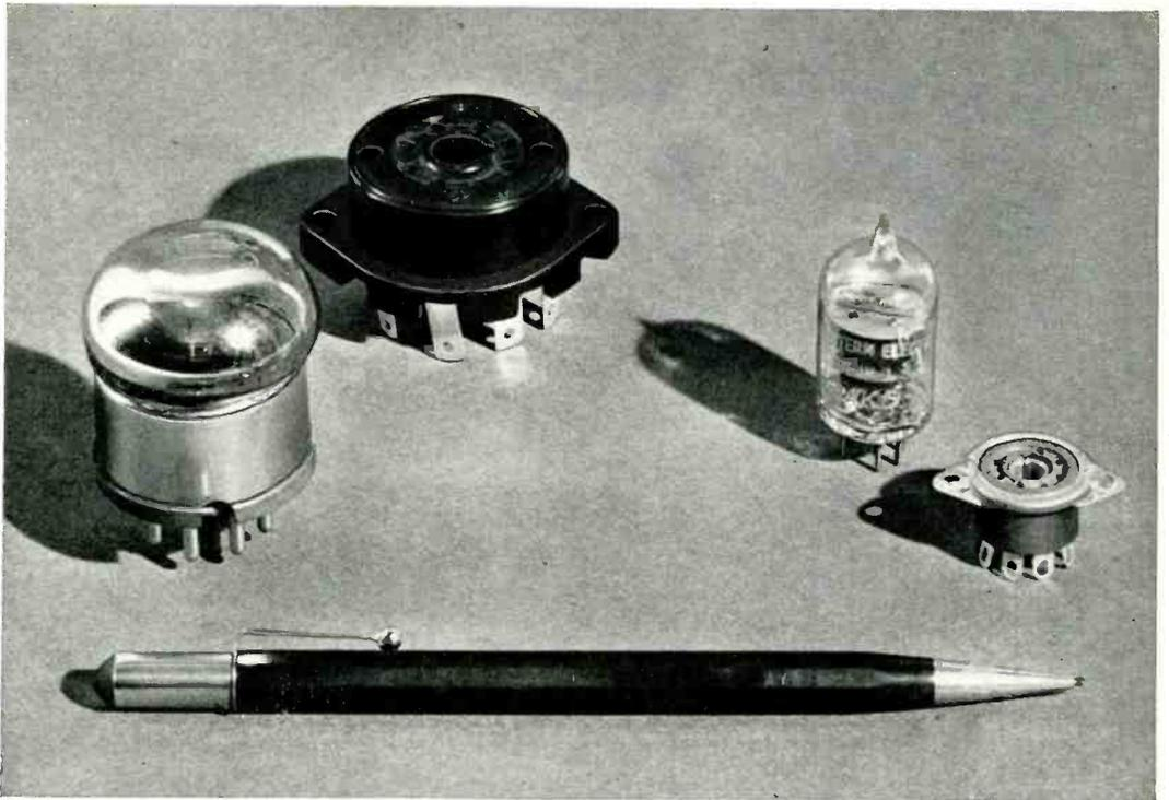
*Fig. 1—Much of the saving in space made possible by the 6AK5 tube, compared to the 717A tube, is due to the difference in size of the sockets required for the two tubes. The 717A is shown at the left and the 6AK5 at the right*
