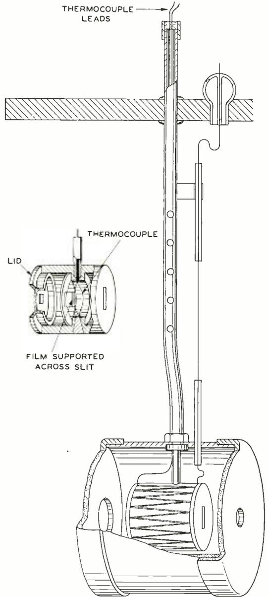
Fig. 7—Electric furnace in which alloy films were heat treated inside the diffraction camera. A heating element of nichrome wire was wound on a copper cylinder within which the film was supported on its molybdenum slit. Temperatures were measured with an iron-constantan thermocouple
