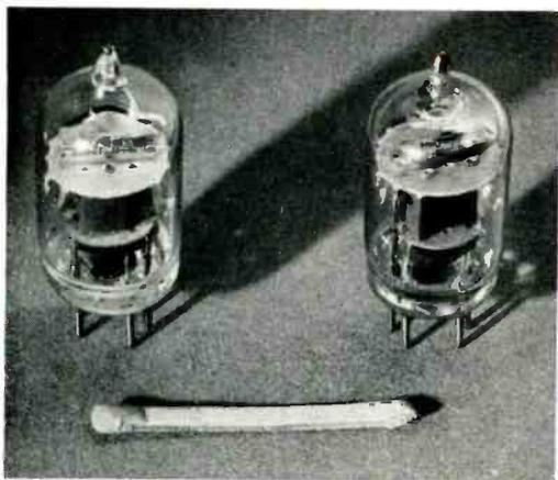
Fig. 4—The 6AJ5 tube (left) is similar in construction to the 6AK5, but is designed particularly for low-power applications in communications equipment for aircraft. The characteristics of the 6AJ5 tube follow:
