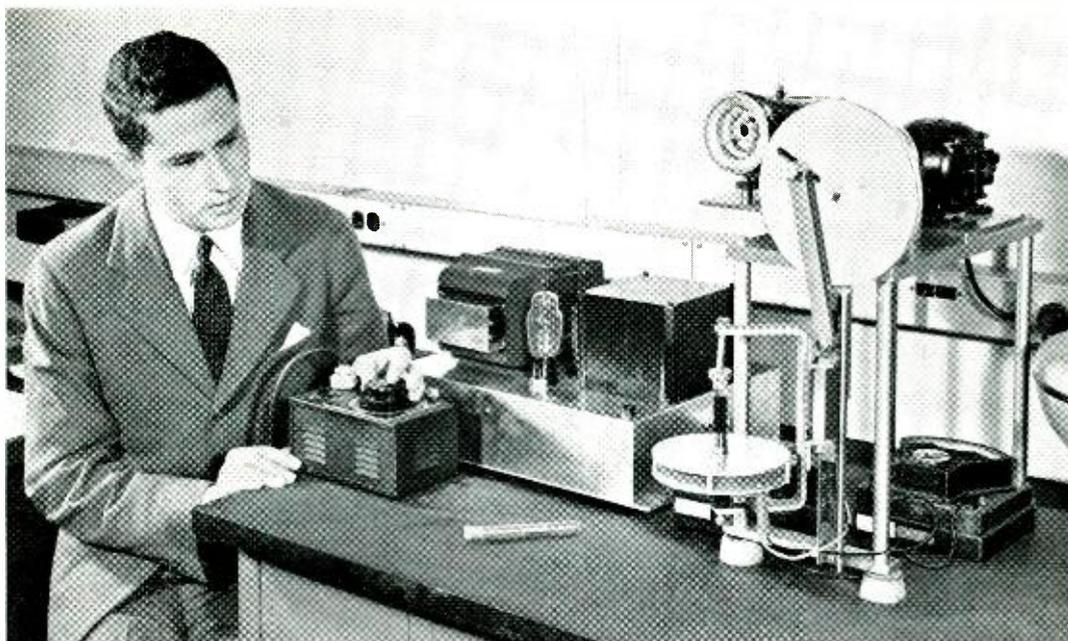
*J. W. Mullen, II, adjusts the current of an electromagnet that operates the plunger of this automatic stirrer*
